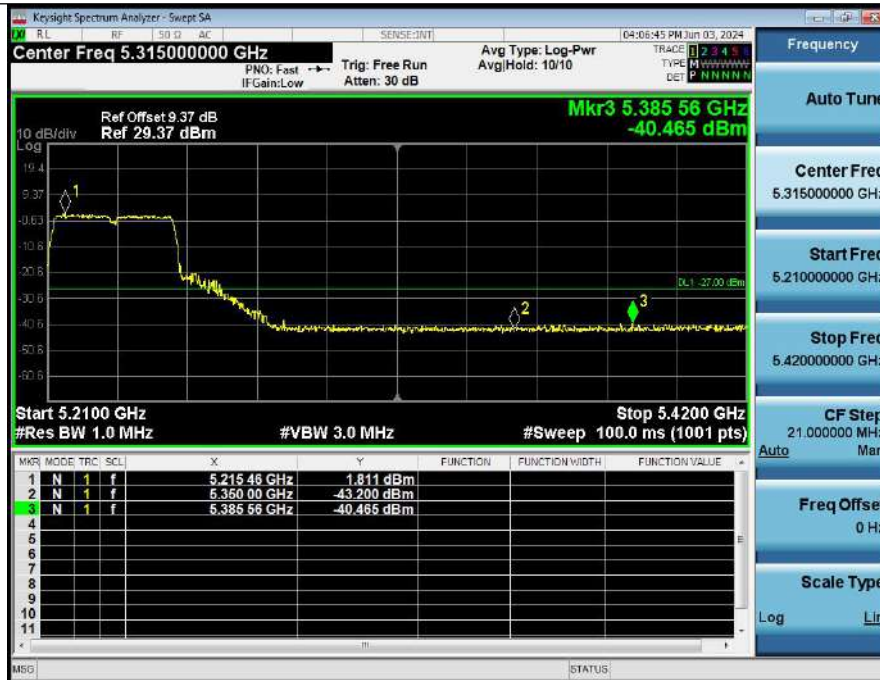
Bandedge_NVNT_ANT1_802_11ac(VHT40)_5190
