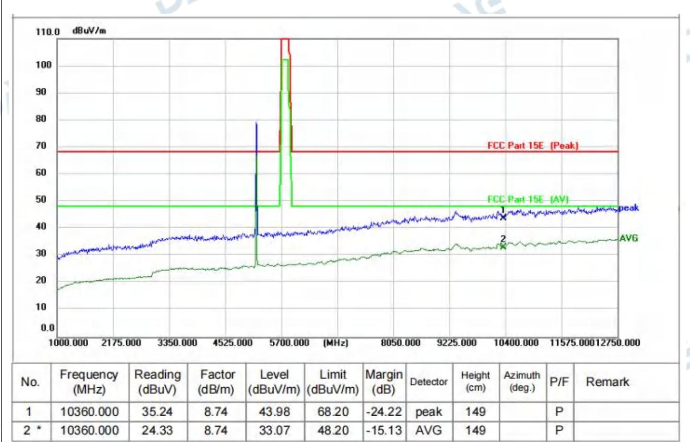
TM1 / Polarization: Vertical / Band: 5150-5250 MHz / BW: 20 / CH: L
