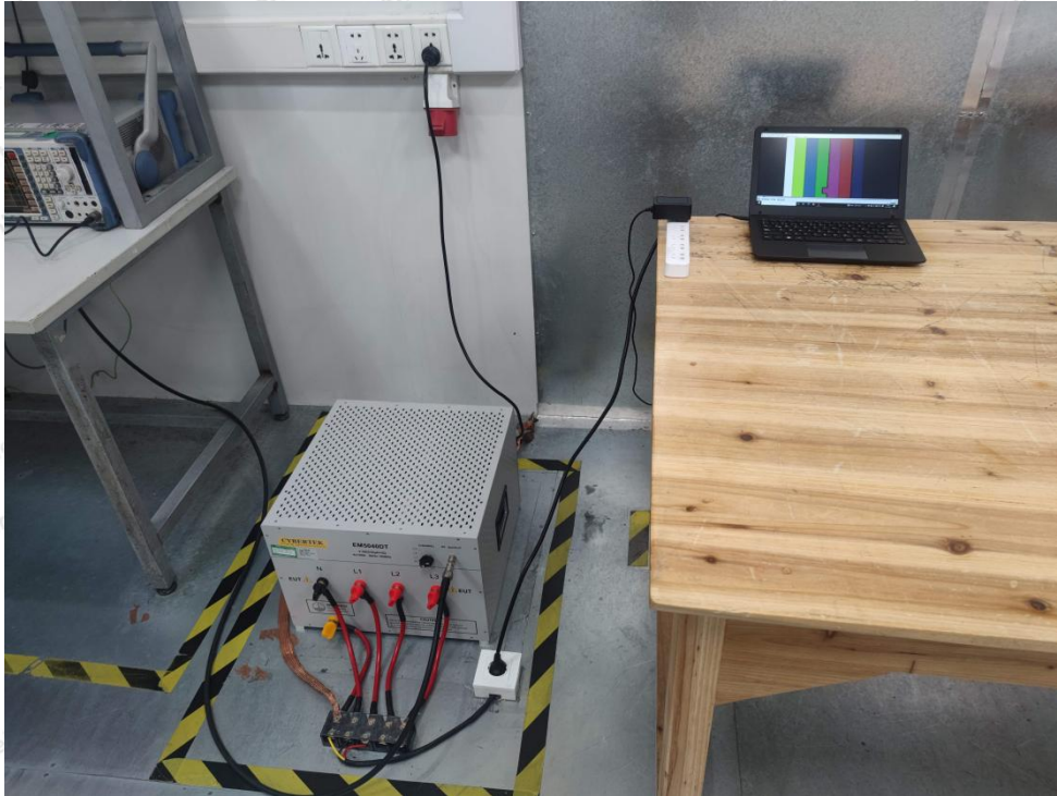
Photo of Power Line Conducted Emission Test
