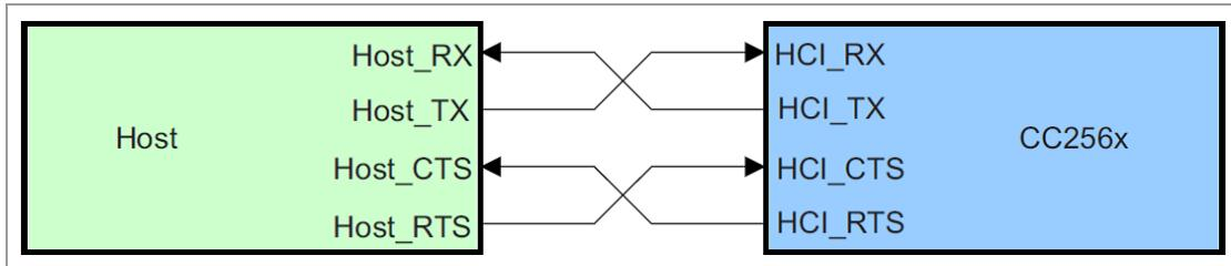
When the UART RX buffer of the CC2564C passes the “flow control” threshold, it will set the signal UART\_RTS high to stop transmission from the host.
