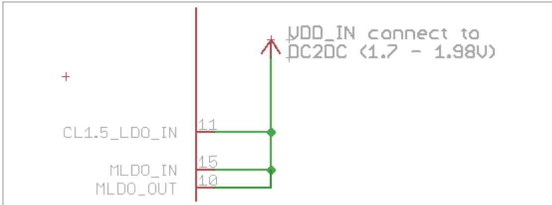
Mixed DC2DC- $V_{BAT}$  system (Maximum RF output power and optimum system power, but requires routing of  $V_{BAT}$ ):
