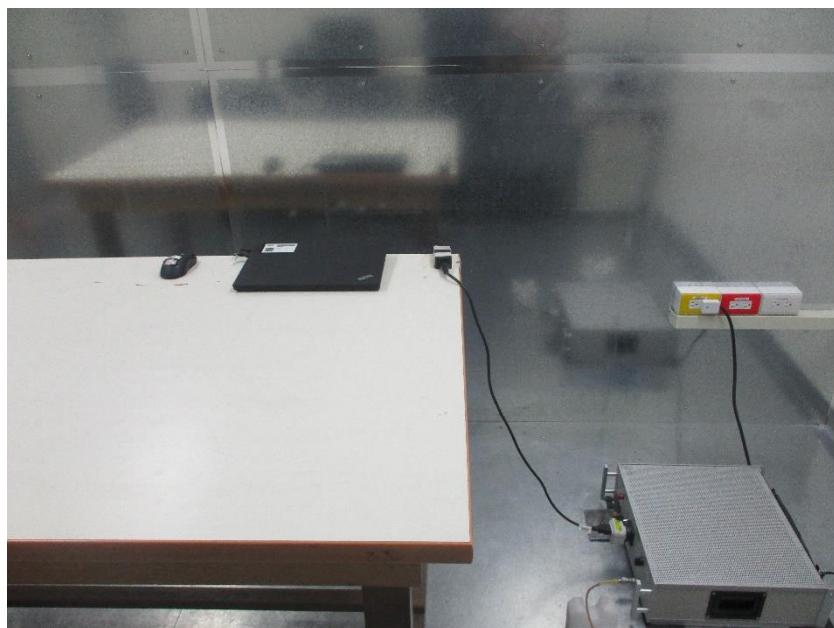
**Conducted Setup Photo (Measurement at Antenna Port)**
