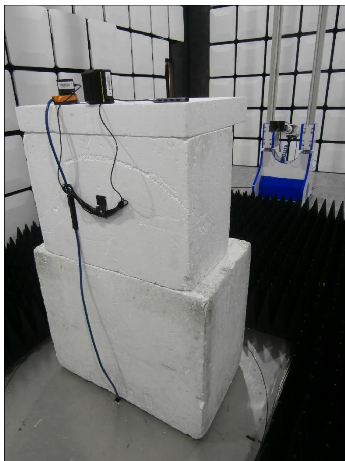
Figure 20 - Test Setup - 1 GHz to 13 GHz - X Orientation
