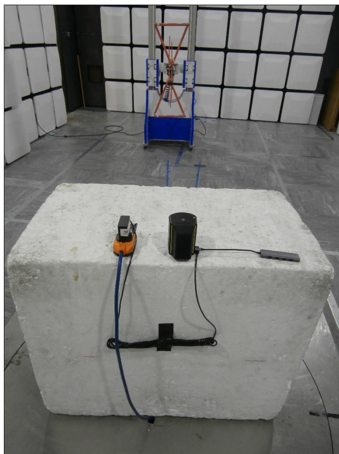
Figure 18 - Test Setup - 30 MHz to 1 GHz - X Orientation
