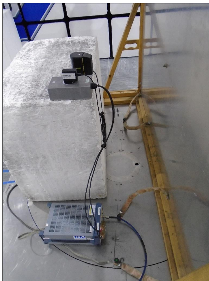
Figure 16 - Test Setup - AC Line Conducted Emissions
