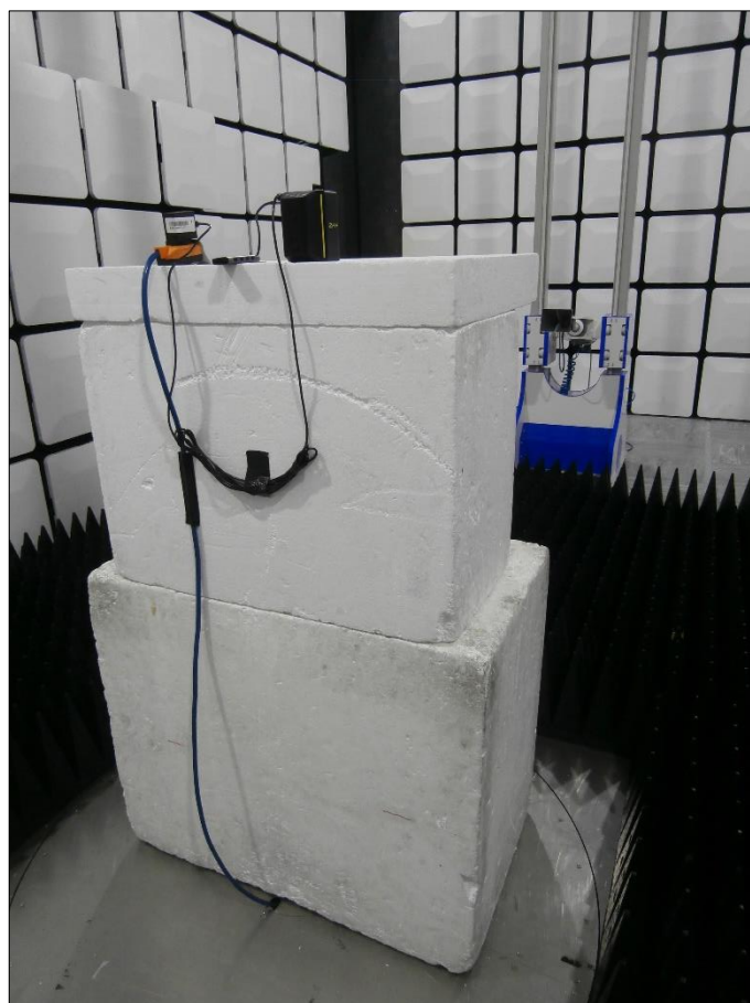
Figure 21 - Test Setup - 1 GHz to 13 GHz - Y Orientation
