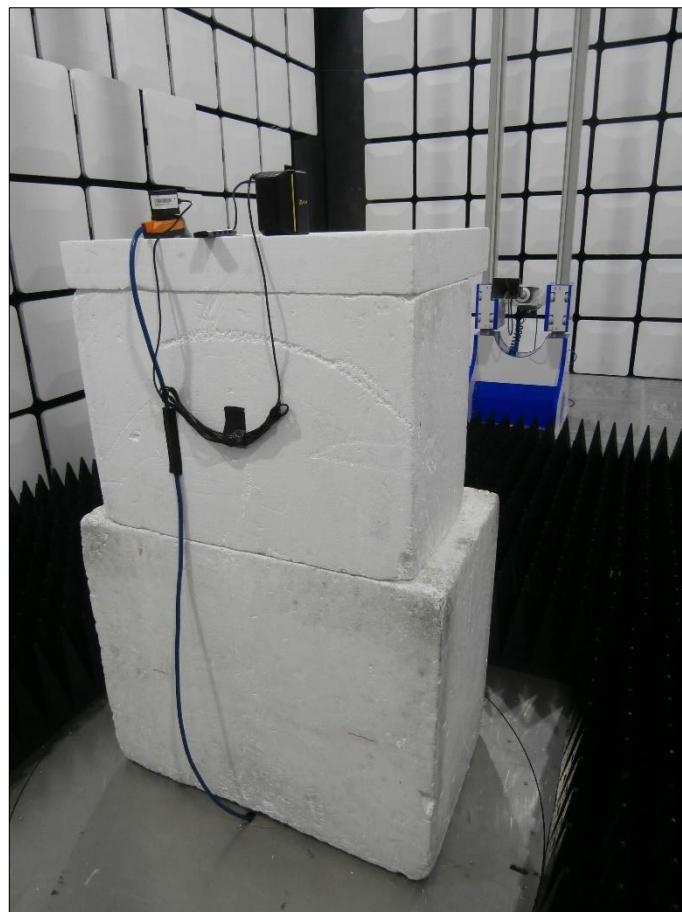
**Figure 6 - Test Setup - 1 GHz to 13 GHz - Y Orientation**
