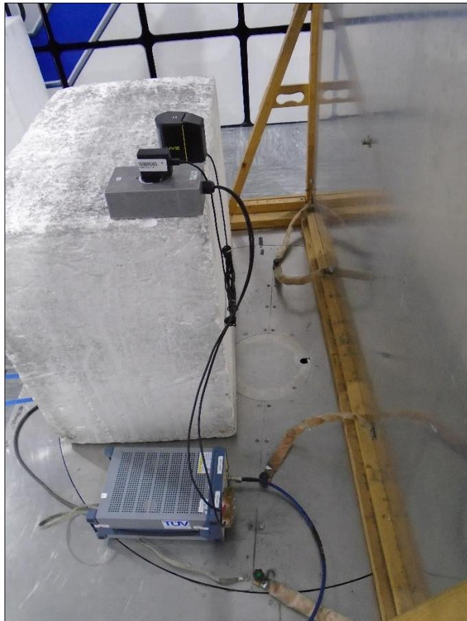
Figure 1 - Test Setup - AC Line Conducted Emissions
