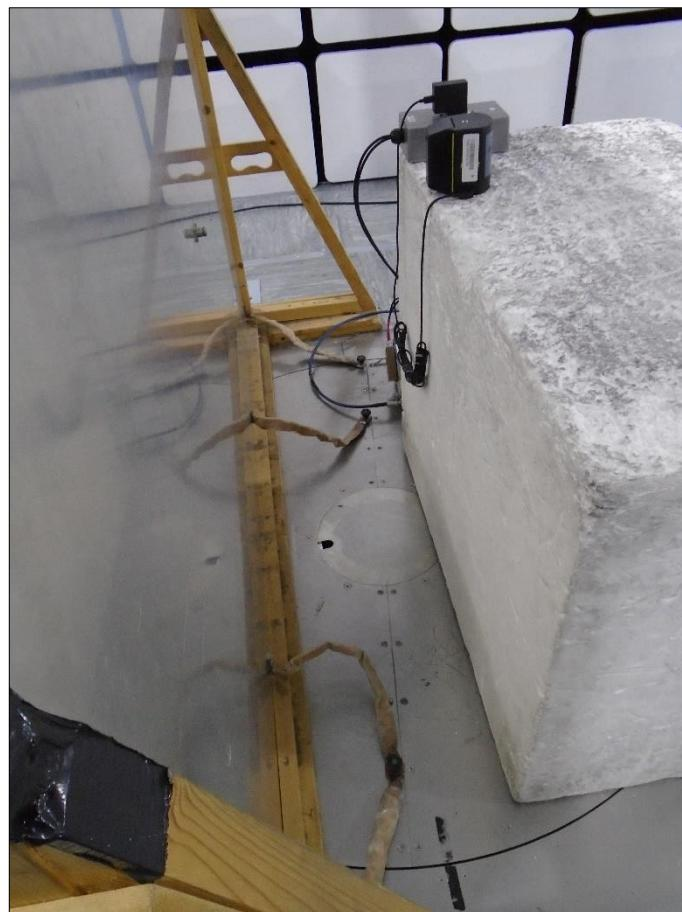
**Figure 2 - Test Setup - AC Line Conducted Emissions**
