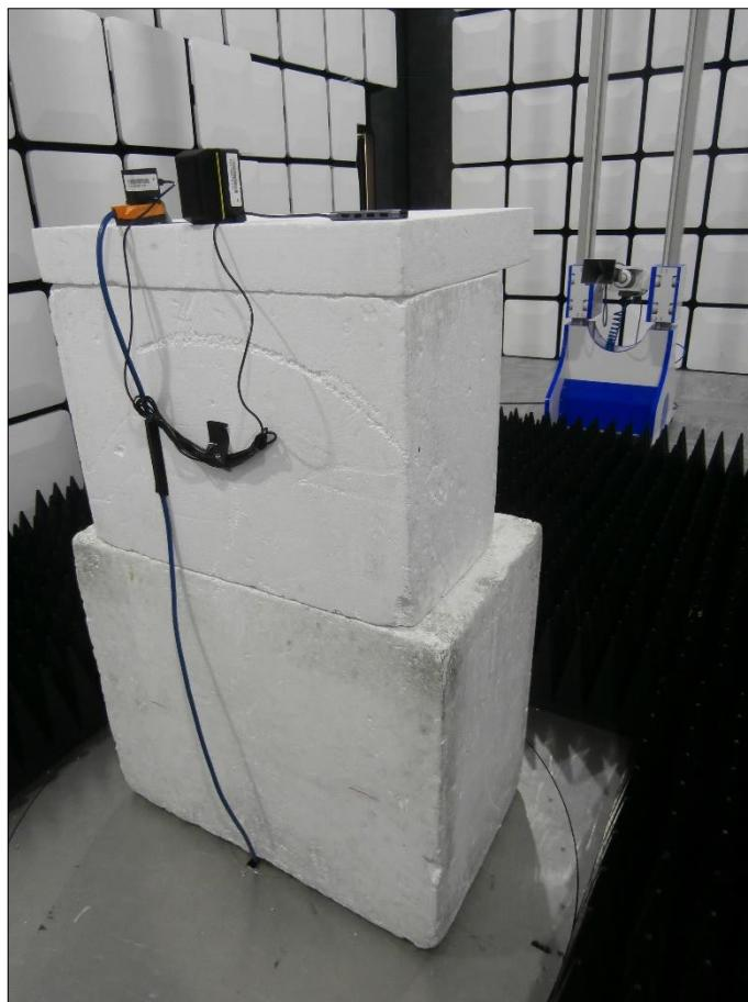
**Figure 5 - Test Setup - 1 GHz to 13 GHz - X Orientation**
