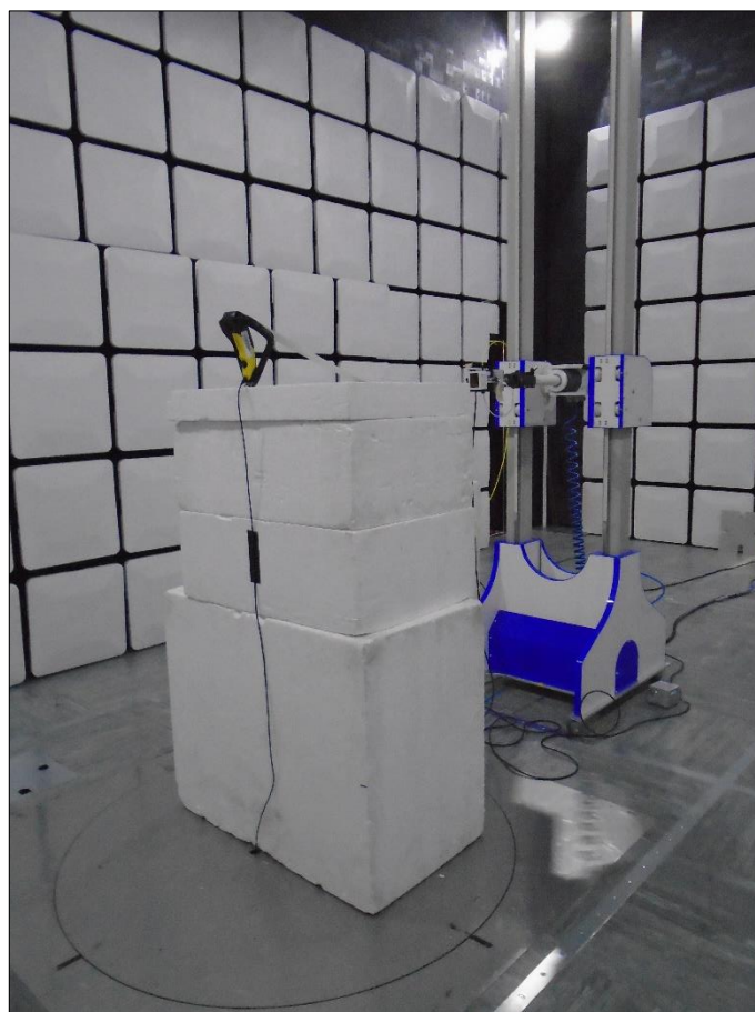
Figure 65 - Test Setup - 18 GHz to 25 GHz - Y Orientation
