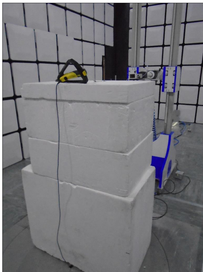
Figure 66 - Test Setup - 18 GHz to 25 GHz - Z Orientation
