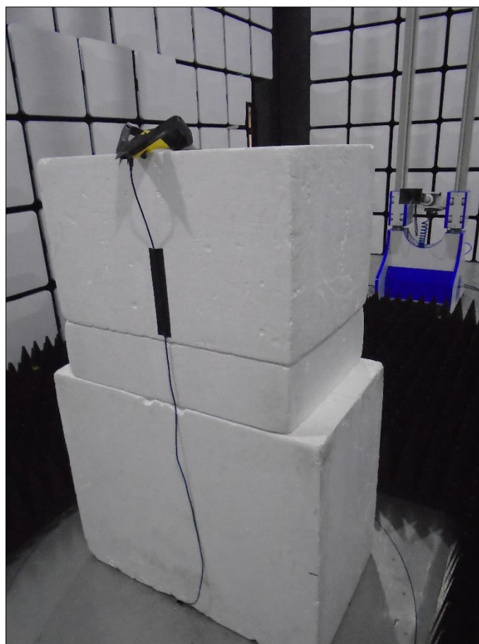
Figure 61 - Test Setup - 1 GHz to 18 GHz - X Orientation
