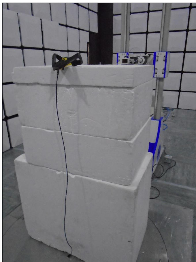
Figure 64 - Test Setup - 18 GHz to 25 GHz - X Orientation
