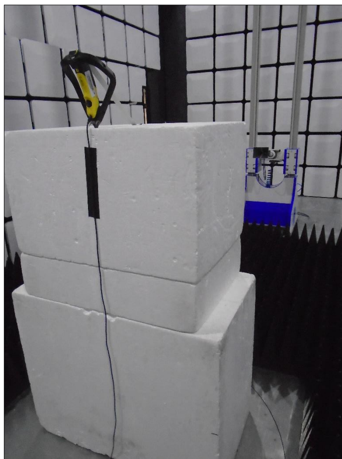
Figure 62 - Test Setup - 1 GHz to 18 GHz - Y Orientation
