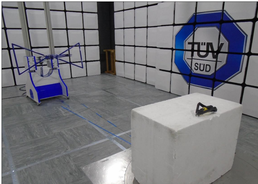
Figure 18 - Test Setup - Below 1 GHz - Y Orientation
