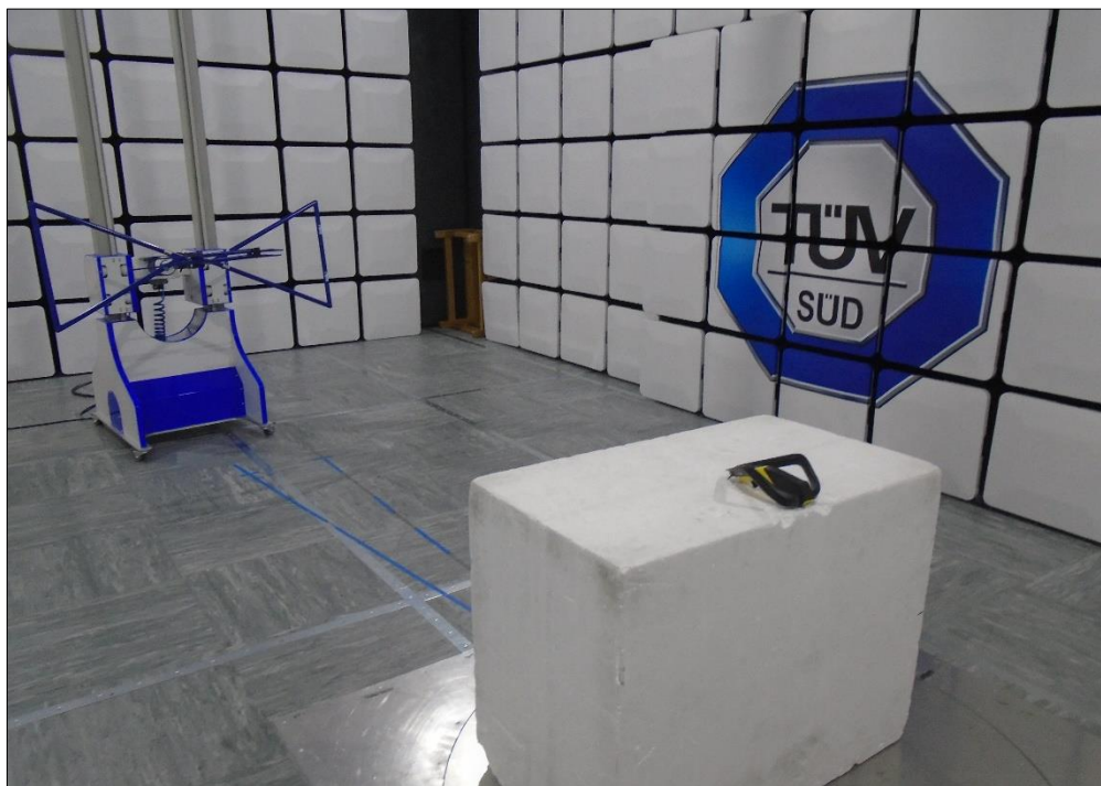
Figure 20 - Test Setup - Below 1 GHz - Z Orientation
