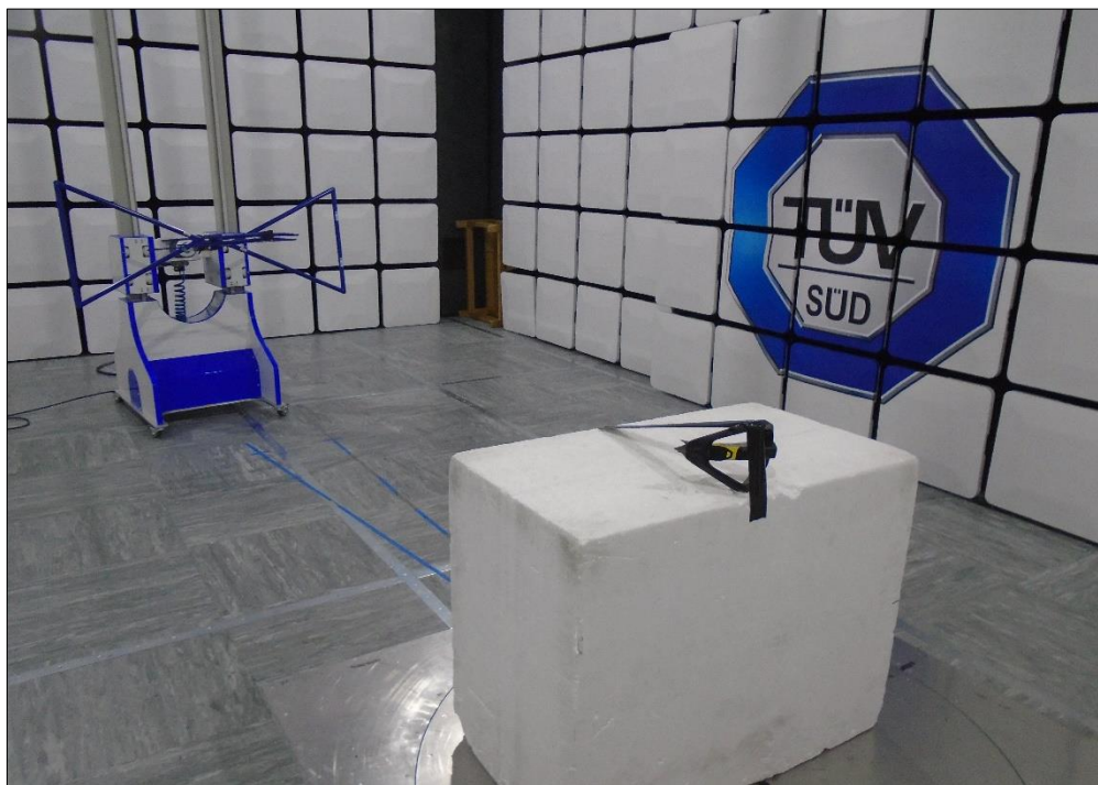
Figure 16- Test Setup - Below 1 GHz - X Orientation
