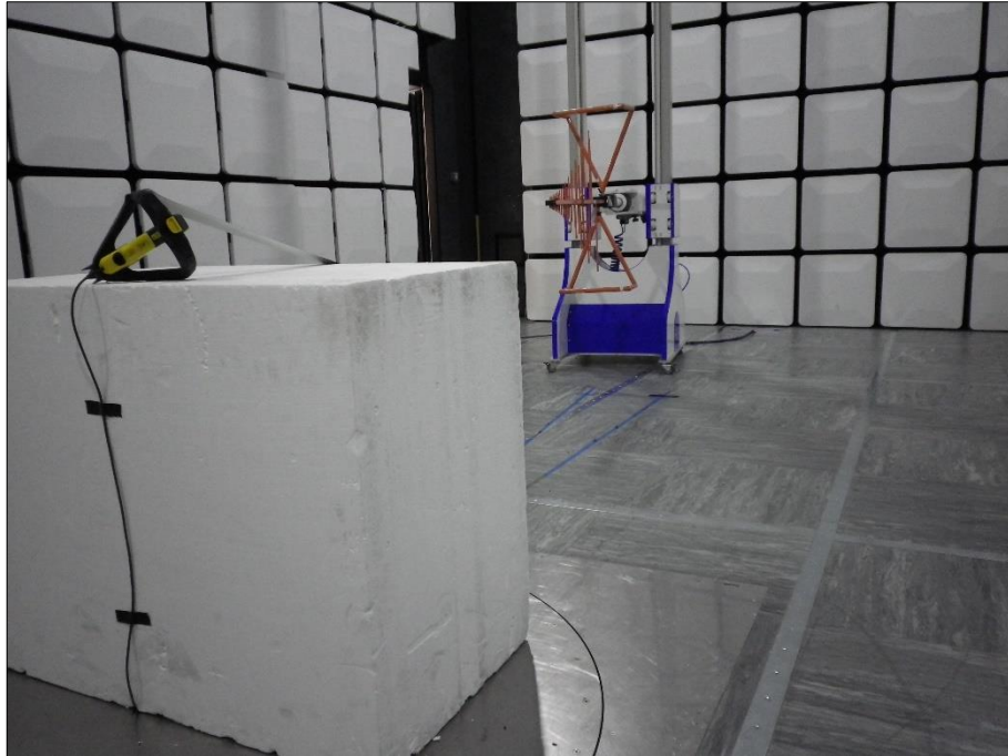
Figure 3 - Test Setup - 30 MHz to 1 GHz - Z Orientation
