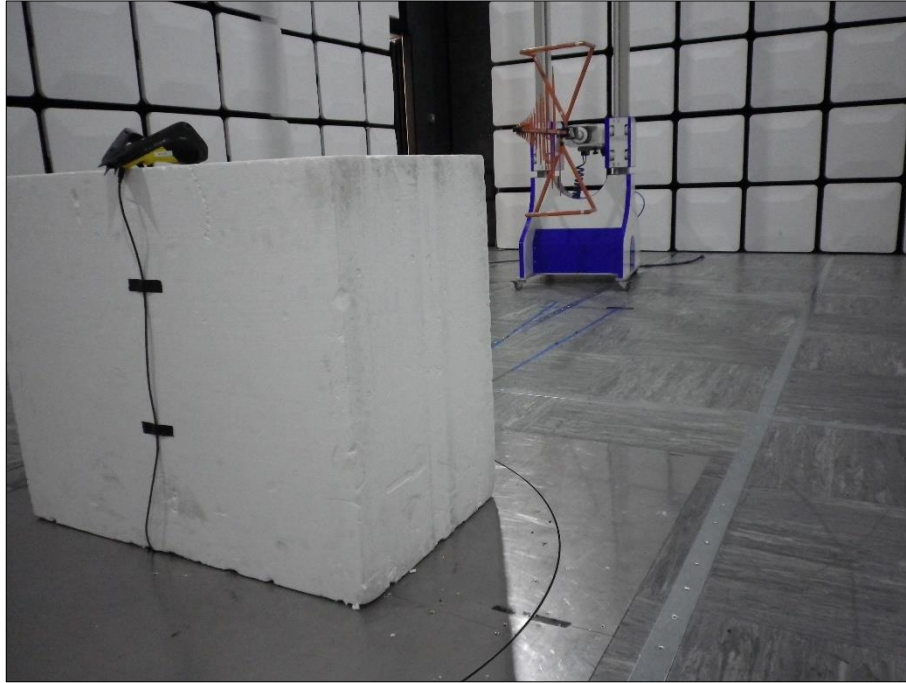
Figure 1 - Test Setup - 30 MHz to 1 GHz - X Orientation
