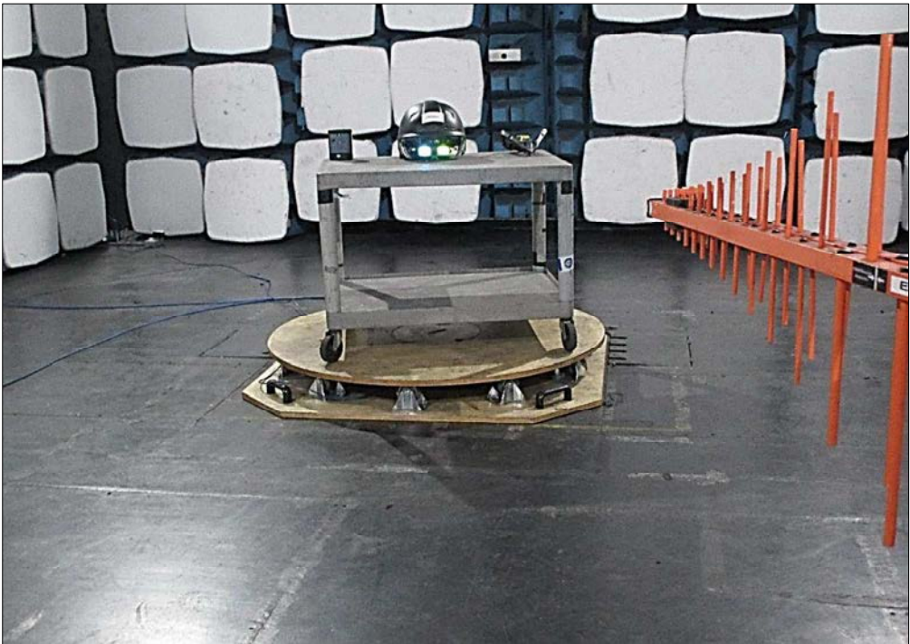
Figure 30 - Test Setup - 30 MHz to 1 GHz - X Orientation
