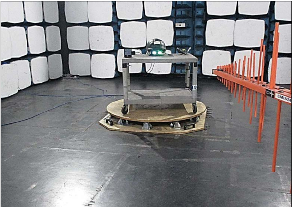
Figure 54 - Test Setup - 30 MHz to 1 GHz - X Orientation
