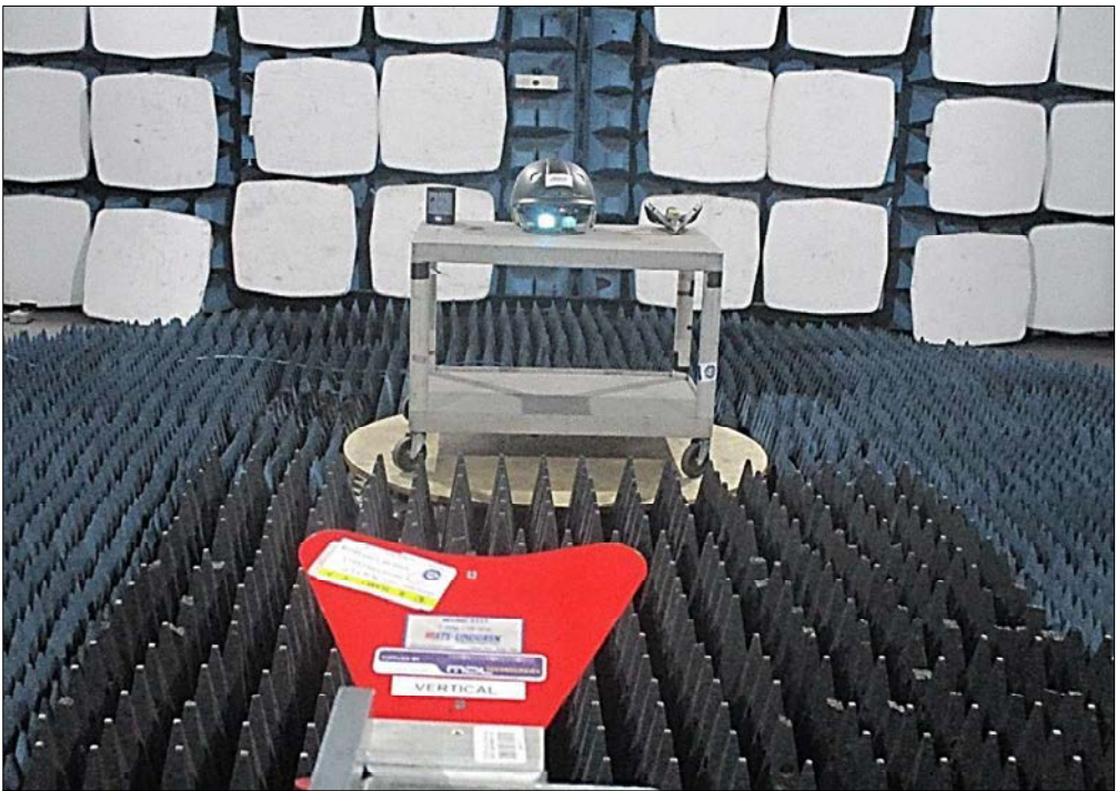
Figure 31 - Test Setup - 1 GHz to 13 GHz- X Orientation
