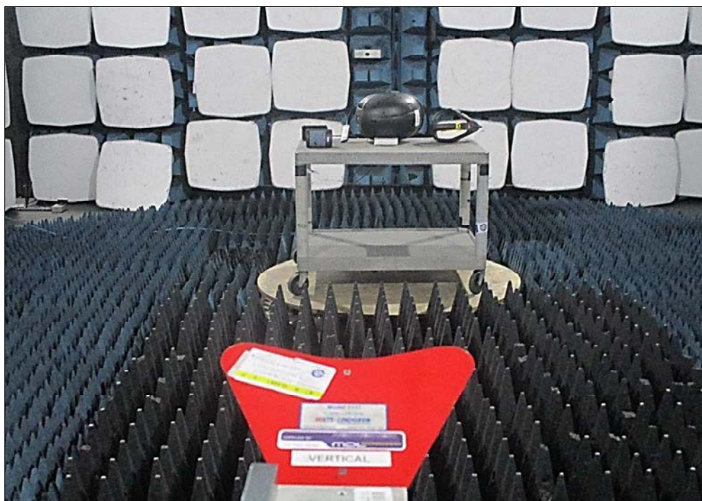
Figure 57 - Test Setup - 1 GHz to 13 GHz - Y Orientation
