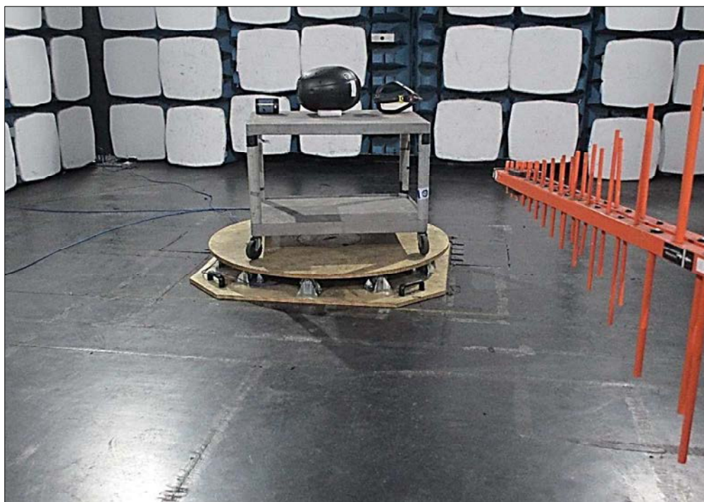
Figure 32 - Test Setup - 30 MHz to 1 GHz- Y Orientation
