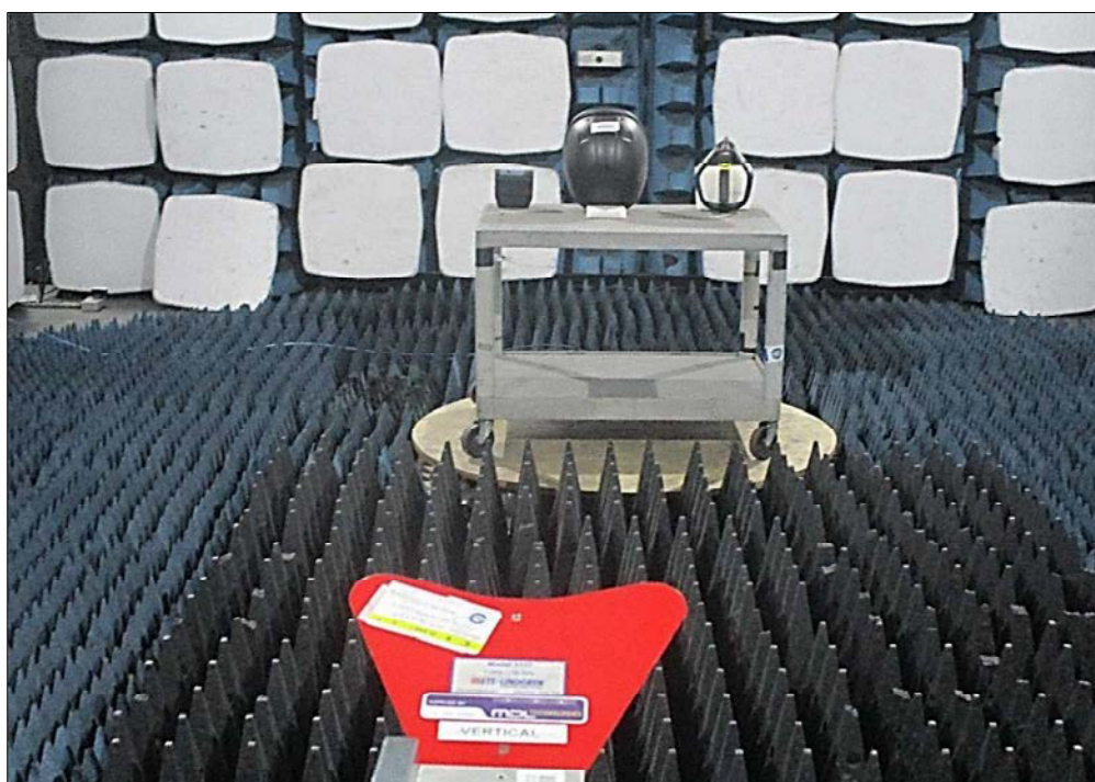
Figure 35 - Test Setup - 1 GHz to 13 GHz- Z Orientation
