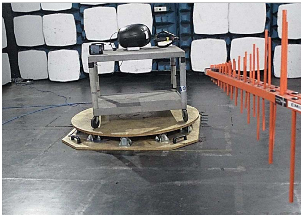
Figure 56 - Test Setup - 30 MHz to 1 GHz - Y Orientation
