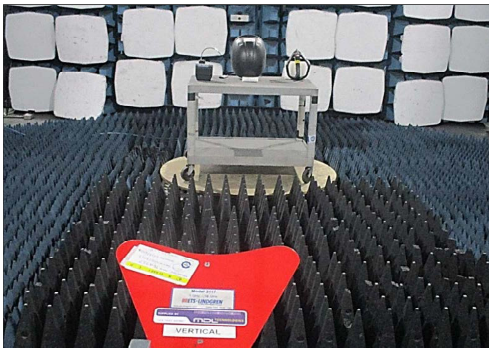
Figure 59 - Test Setup - 1 GHz to 18 GHz - Z Orientation
