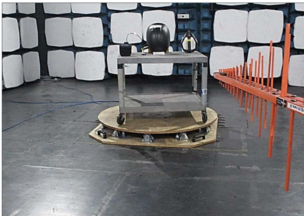
Figure 58 - Test Setup - 30 MHz to 1 GHz - Z Orientation
