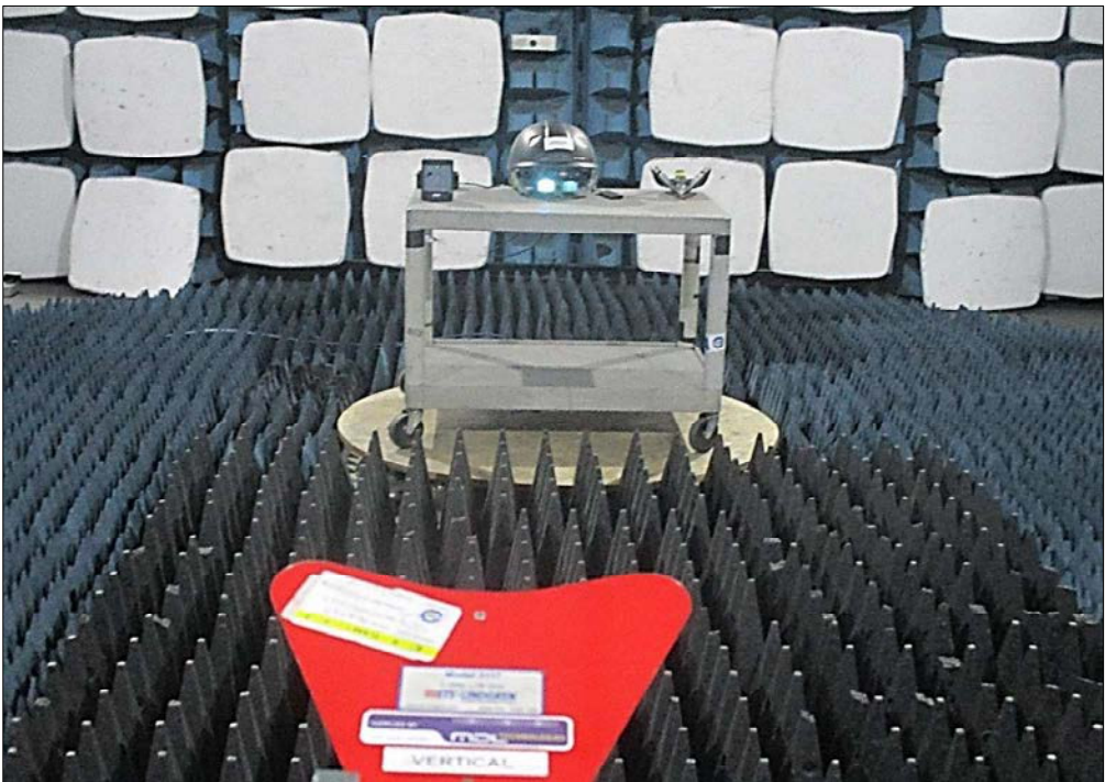
Figure 55 - Test Setup - 1 GHz to 13 GHz - X Orientation
