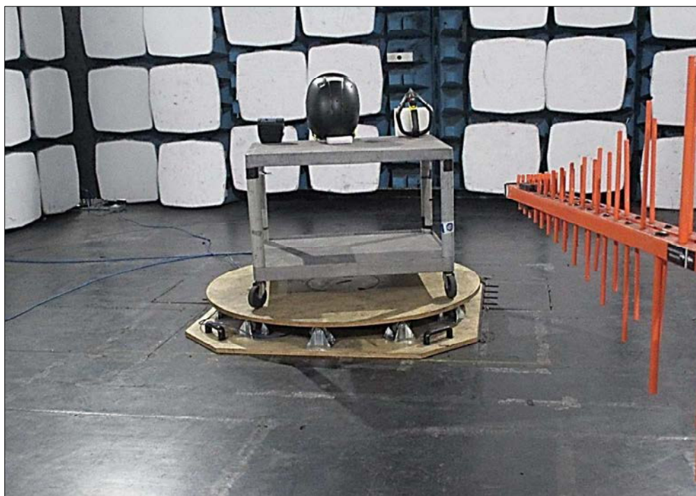
Figure 34 - Test Setup - 30 MHz to 1 GHz- Z Orientation
