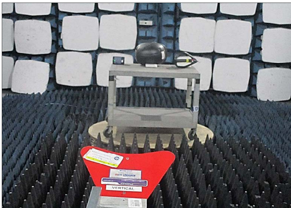
Figure 33 - Test Setup - 1 GHz to 13 GHz- Y Orientation
