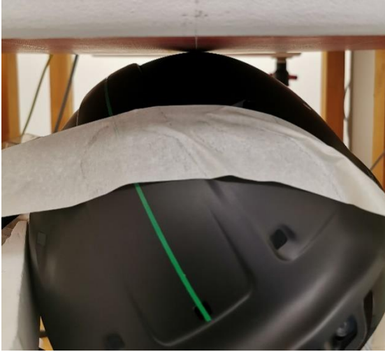
Figure 2 DUT in Left Test Position, 0mm separation distance
