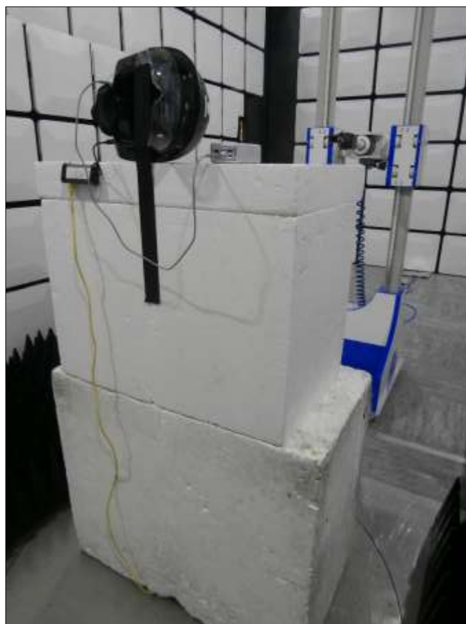
Figure 268 - Test Setup - 18 GHz to 25 GHz - Z Orientation
