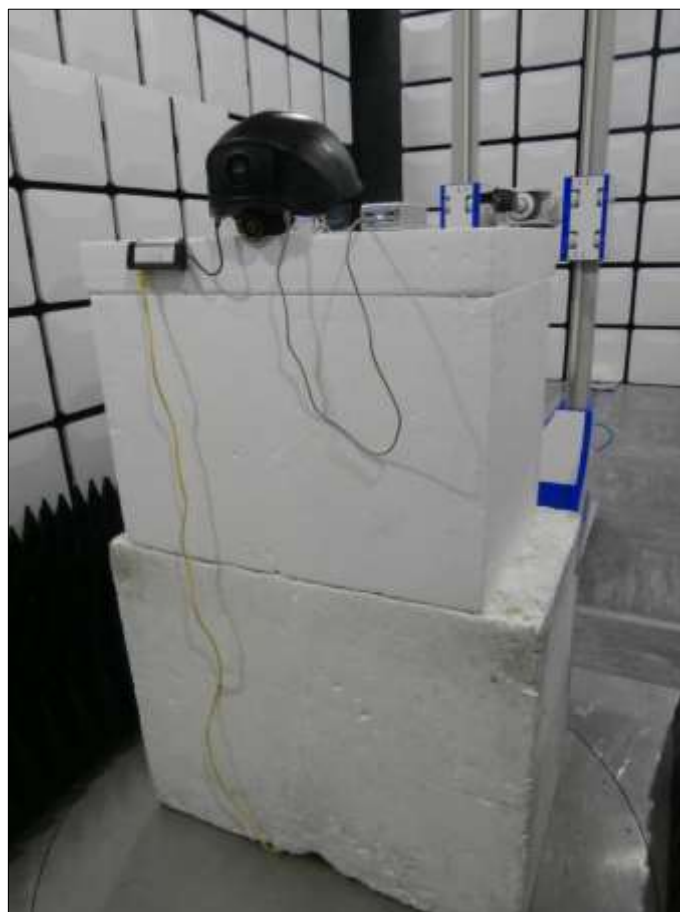
Figure 78 - Test Setup - 18 GHz to 25 GHz - X Orientation
