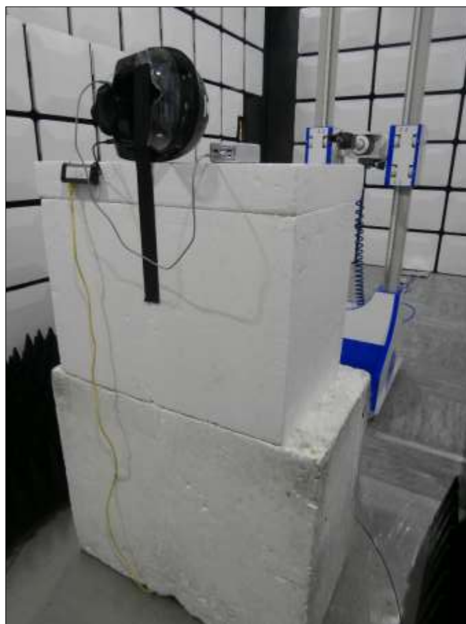
Figure 80 - Test Setup - 18 GHz to 25 GHz - Z Orientation
