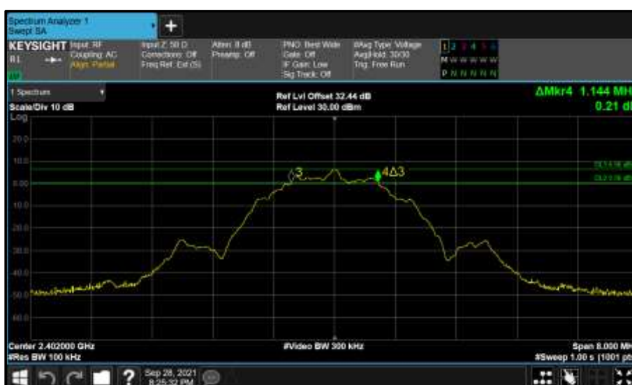
Figure 10 - A (A) 2402 MHz (CH37) 6 dB Bandwidth
