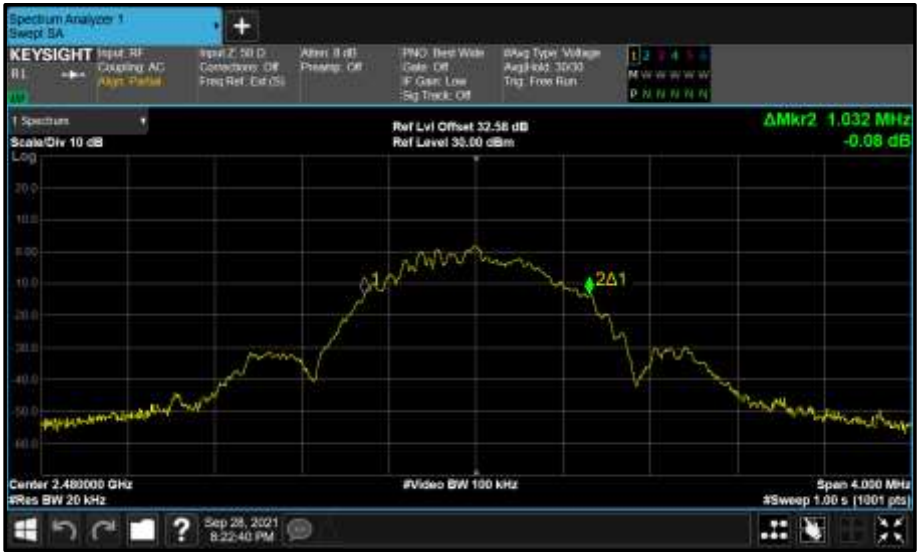
Figure 7 - A (A) 2480 MHz (CH39) 99% Bandwidth
