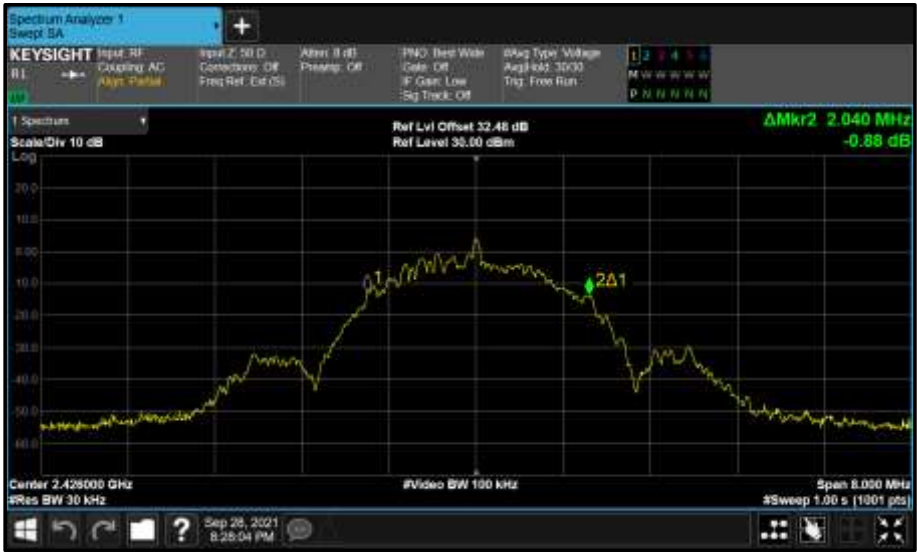
Figure 11 - A (A) 2426 MHz (CH38) 99% Bandwidth
