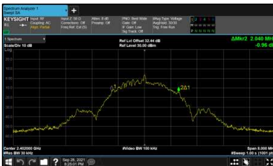
Figure 9 - A (A) 2402 MHz (CH37) 99% Bandwidth
