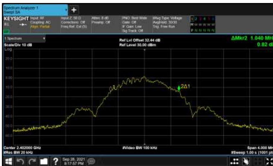
Figure 3 - A (A) 2402 MHz (CH37) 99% Bandwidth
