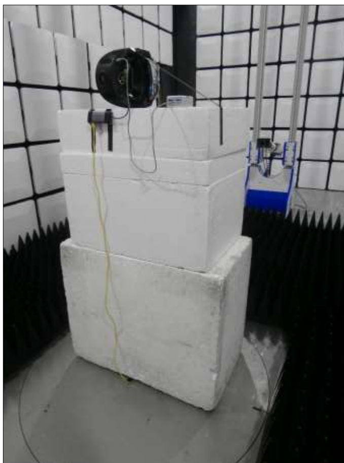
Figure 77 - Test Setup - 1 GHz to 18 GHz - Z Orientation
