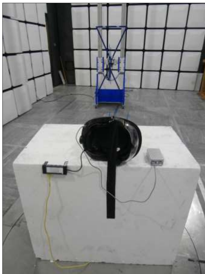
Figure 74 - Test Setup - 30 MHz to 1 GHz - Z Orientation
