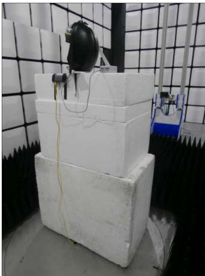
Figure 76 - Test Setup - 1 GHz to 18 GHz - Y Orientation
