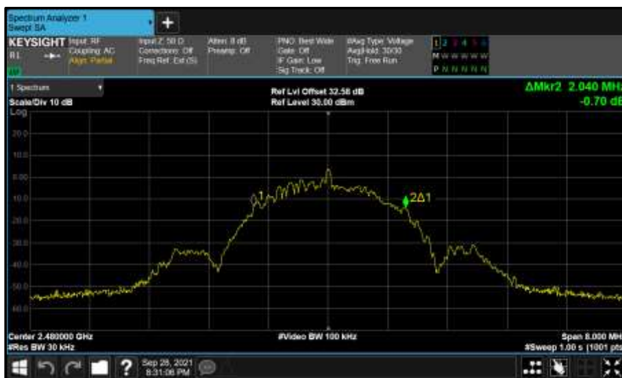
Figure 13 - A (A) 2480 MHz (CH39) 99% Bandwidth
