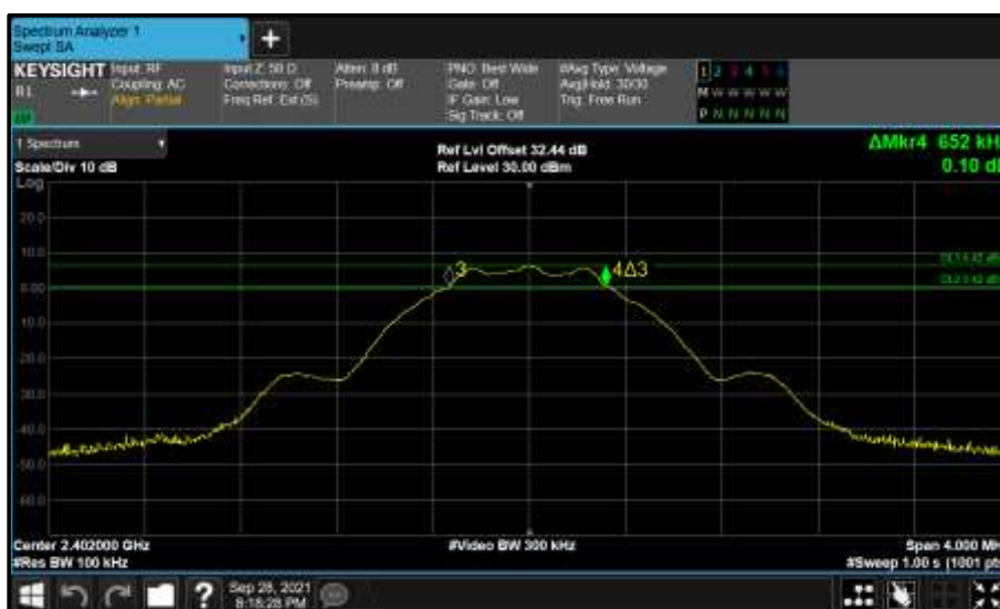
Figure 4 - A (A) 2402 MHz (CH37) 6 dB Bandwidth
