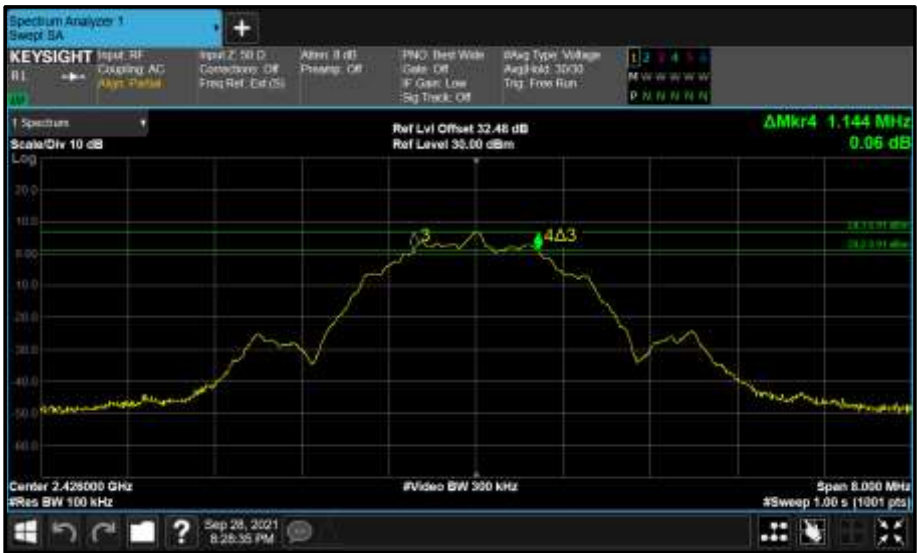
Figure 12 - A (A) 2426 MHz (CH38) 6 dB Bandwidth
