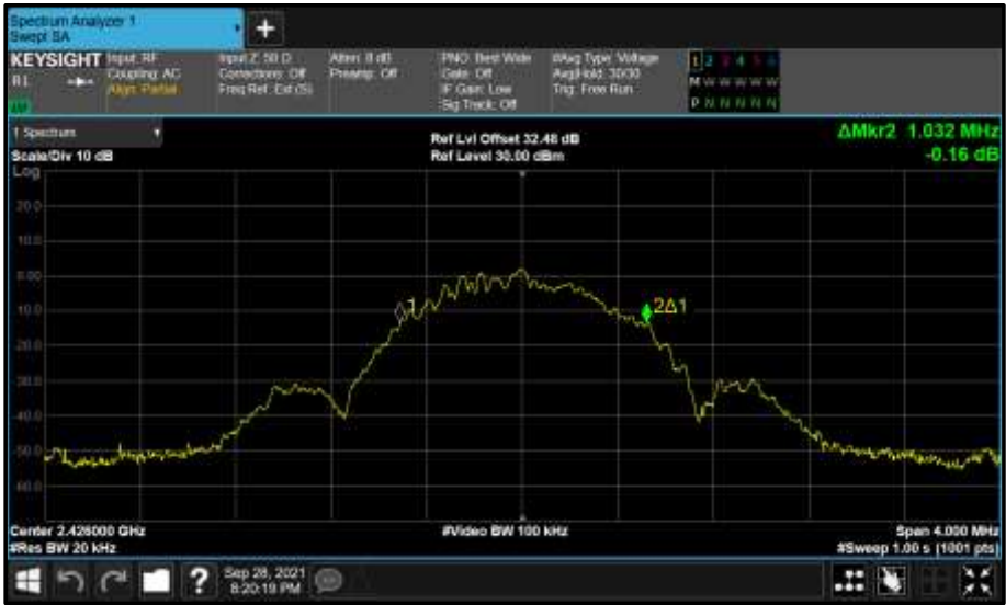
Figure 5 - A (A) 2426 MHz (CH38) 99% Bandwidth
