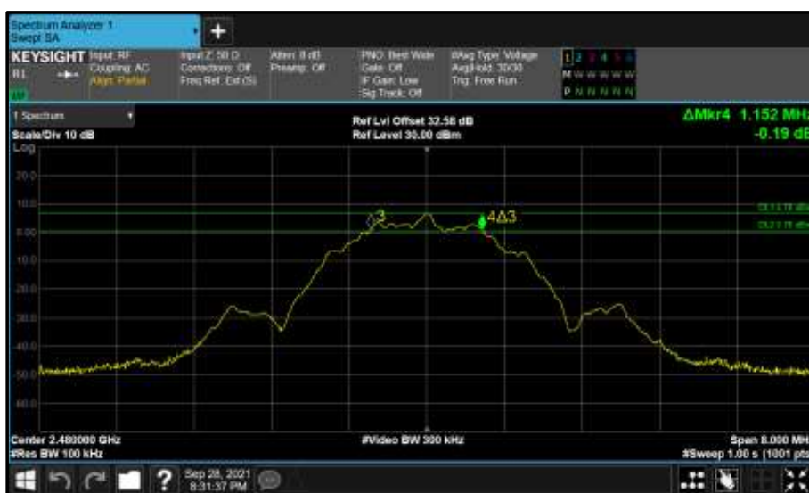
Figure 14 - A (A) 2480 MHz (CH39) 6 dB Bandwidth
