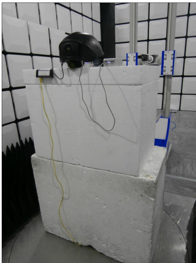
Figure 26 - Test Setup - 18 GHz to 25 GHz - X Orientation
