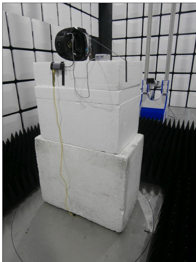
Figure 25 - Test Setup - 1 GHz to 18 GHz - Z Orientation
