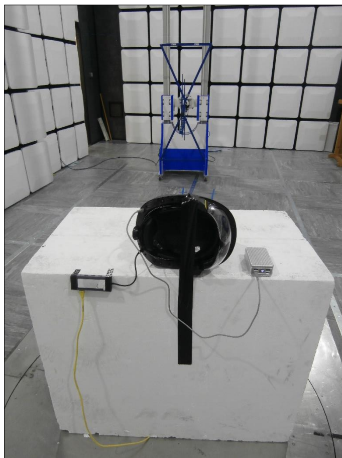
Figure 22 - Test Setup - 30 MHz to 1 GHz - Z Orientation
