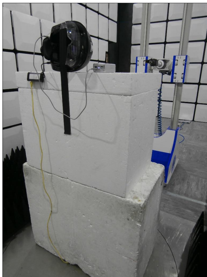
Figure 28 - Test Setup - 18 GHz to 25 GHz - Z Orientation
