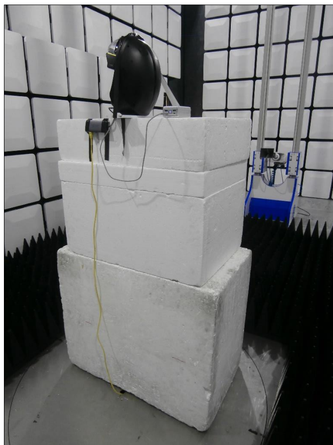
Figure 24 - Test Setup - 1 GHz to 18 GHz - Y Orientation
