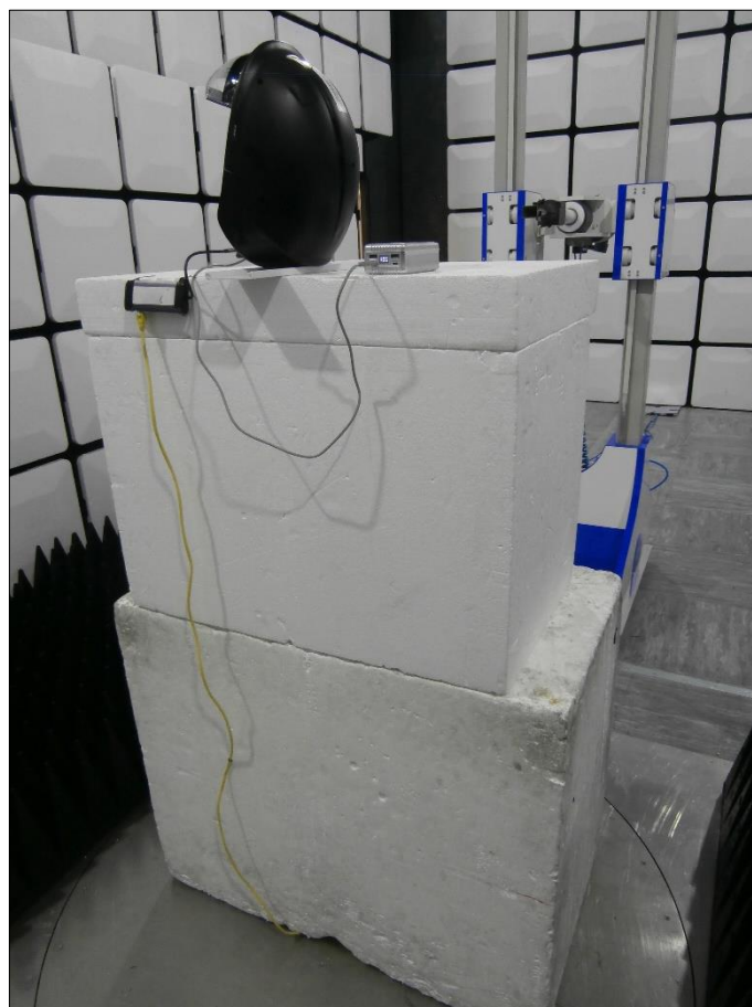
Figure 27 - Test Setup - 18 GHz to 25 GHz - Y Orientation
