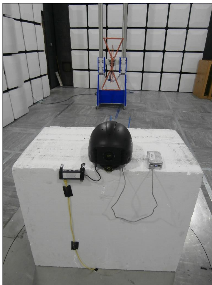
Figure 20 - Test Setup - 30 MHz to 1 GHz - X Orientation
