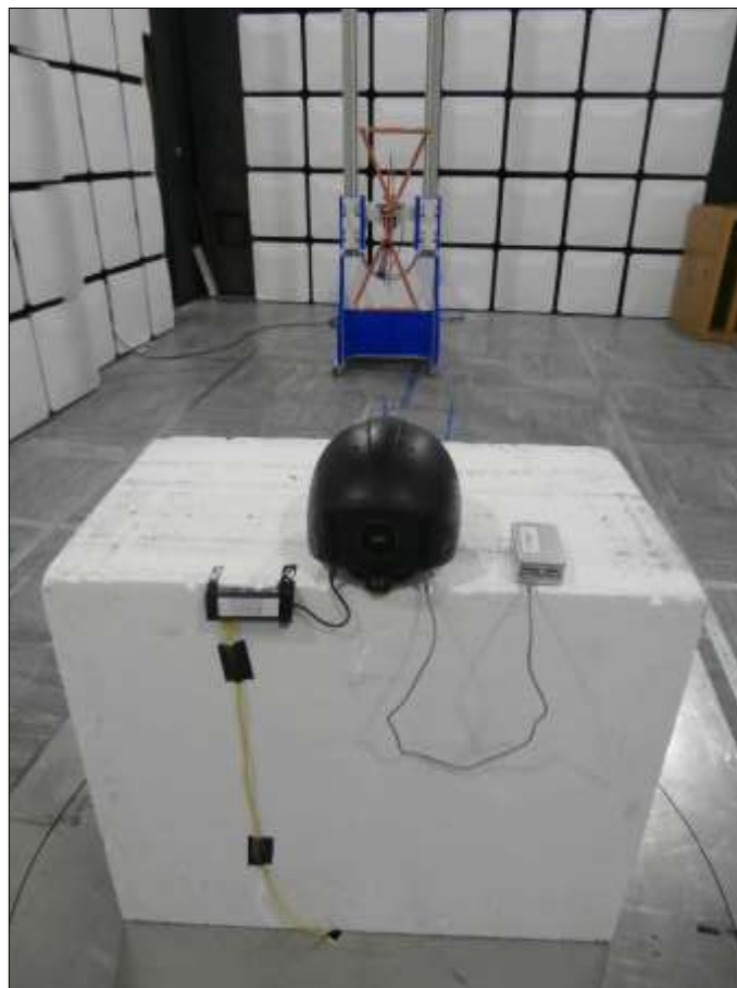
Figure 92 - Test Setup - 30 MHz to 1 GHz - X Orientation
