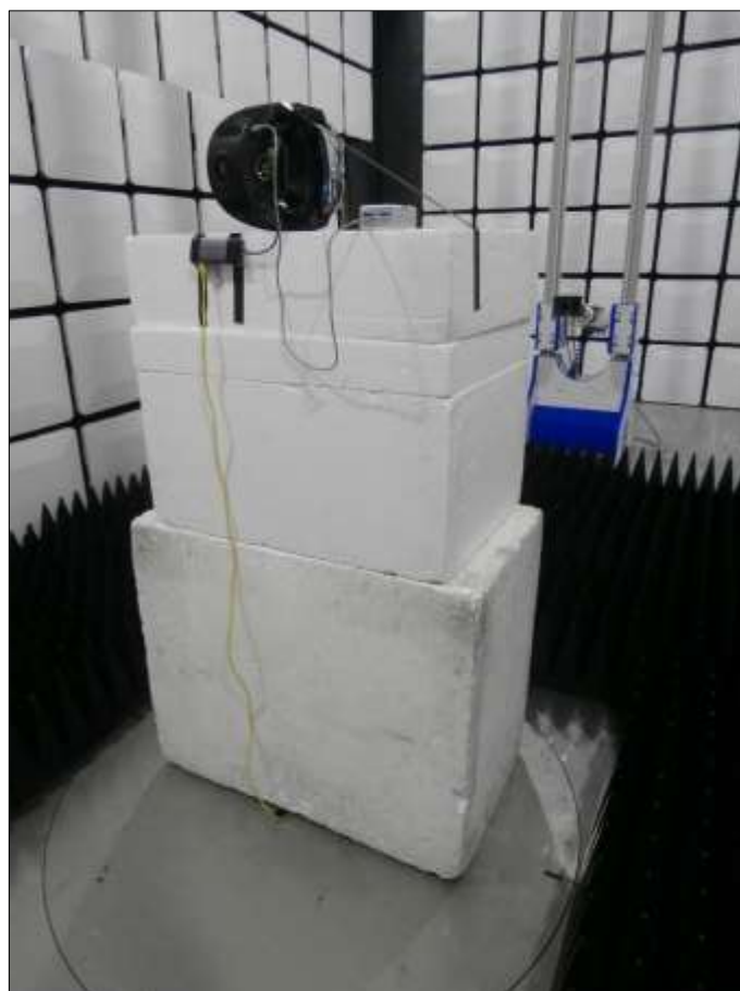
Figure 97 - Test Setup - 1 GHz to 18 GHz - Z Orientation
