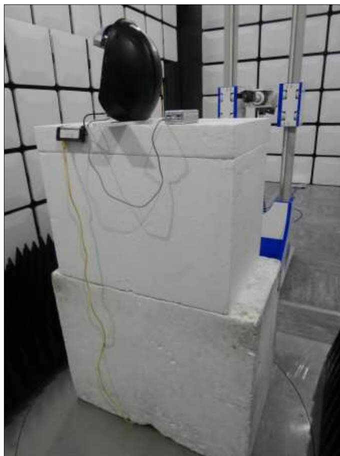
Figure 99 - Test Setup - 18 GHz to 25 GHz - Y Orientation
