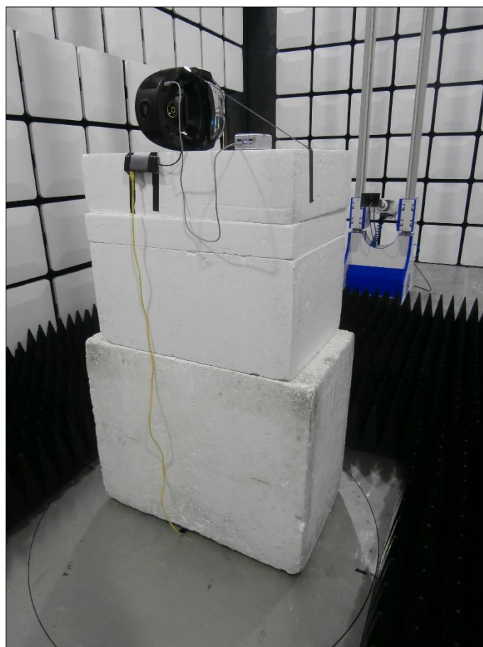
Figure 76 - Test Setup - 1 GHz to 18 GHz - Z Orientation
