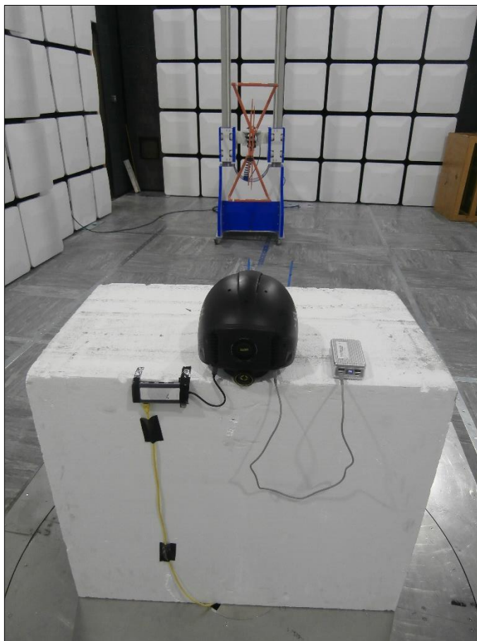
Figure 71 - Test Setup - 30 MHz to 1 GHz - X Orientation
