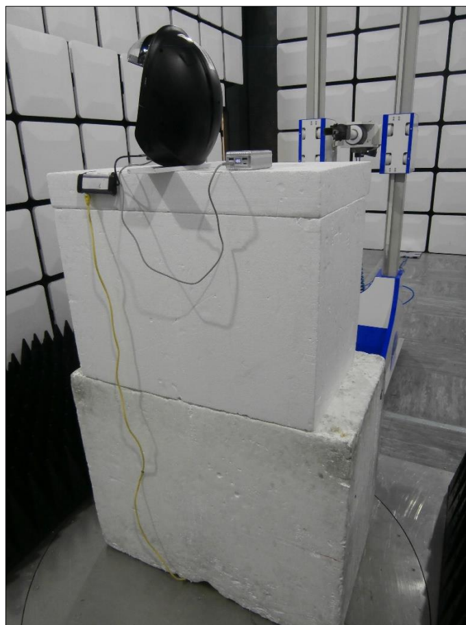
Figure 78 - Test Setup - 18 GHz to 25 GHz - Y Orientation
