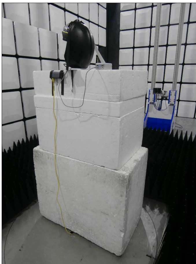
Figure 75 - Test Setup - 1 GHz to 18 GHz - Y Orientation
