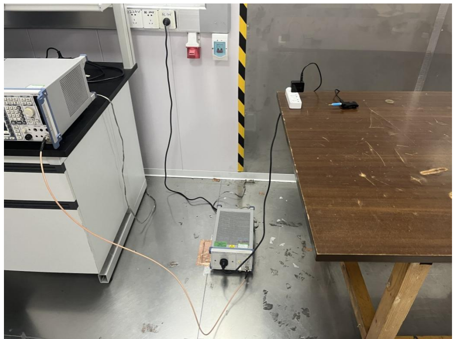
Conducted Emission Test Setup
