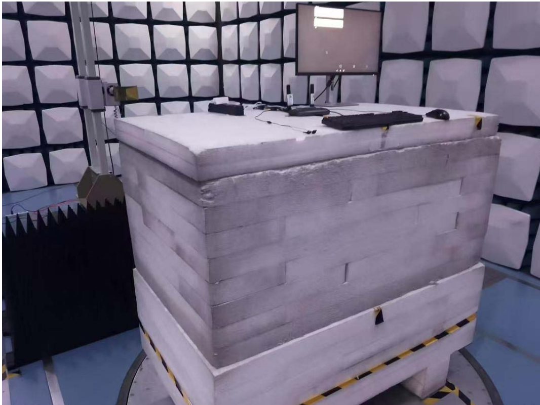
Radiated Emission 18-26.5GHz View
