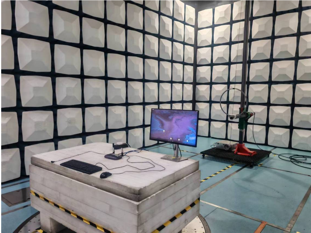
Radiated Emission 9k-30MHz Perpendicular View
