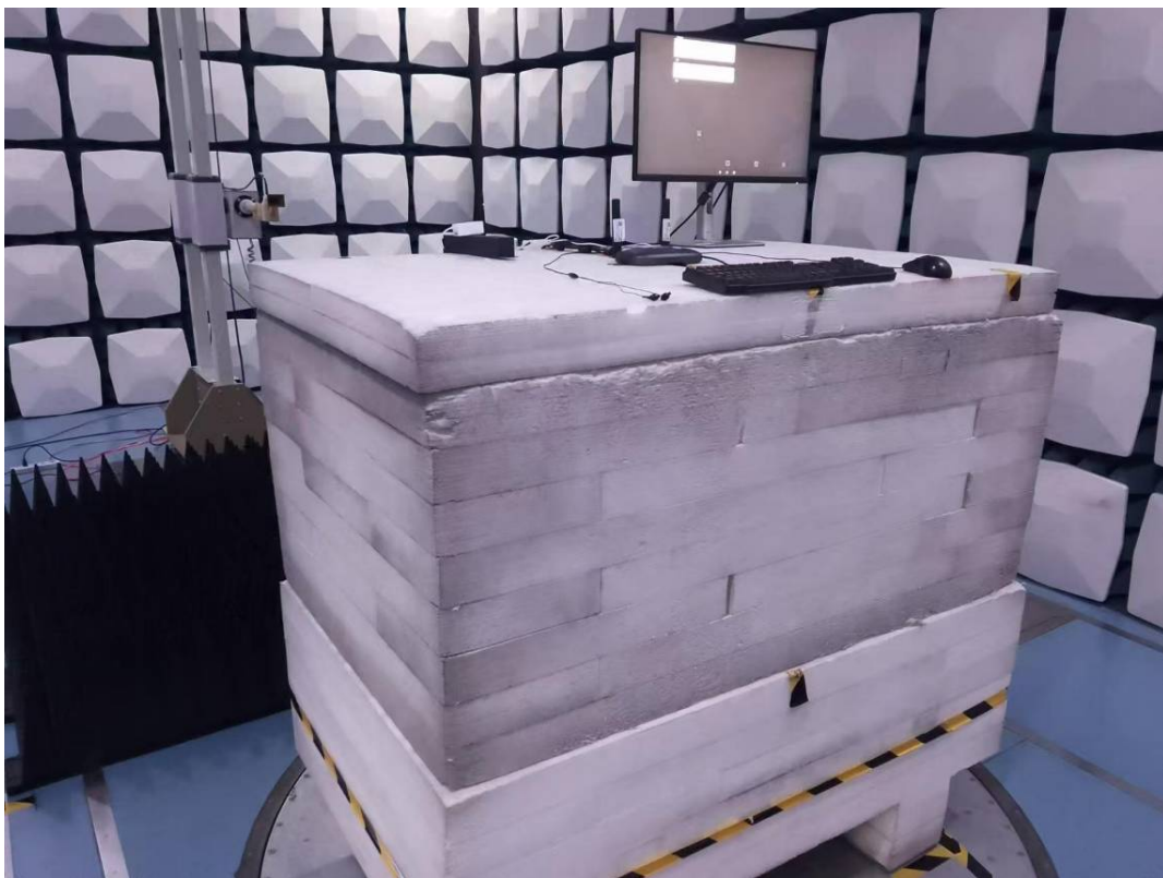
Radiated Emission 18-26.5GHz View
