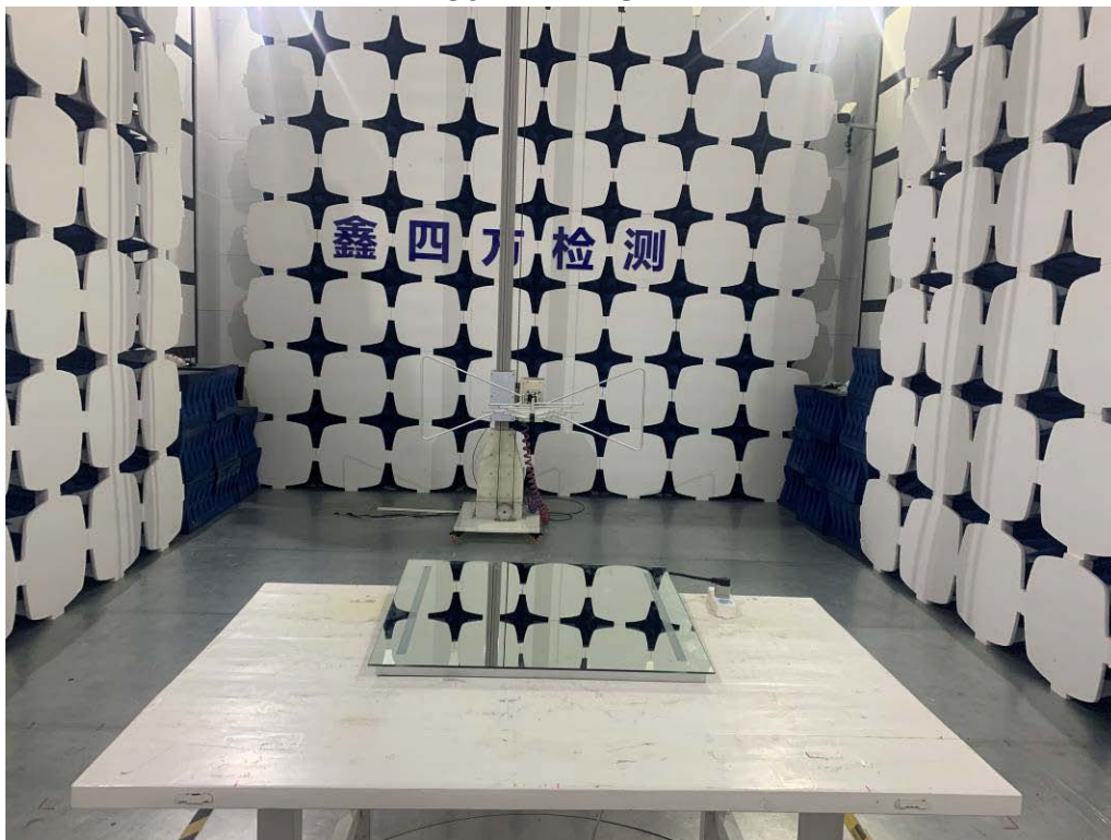
Photos of radiated emission test 30MHz – 1GHz
