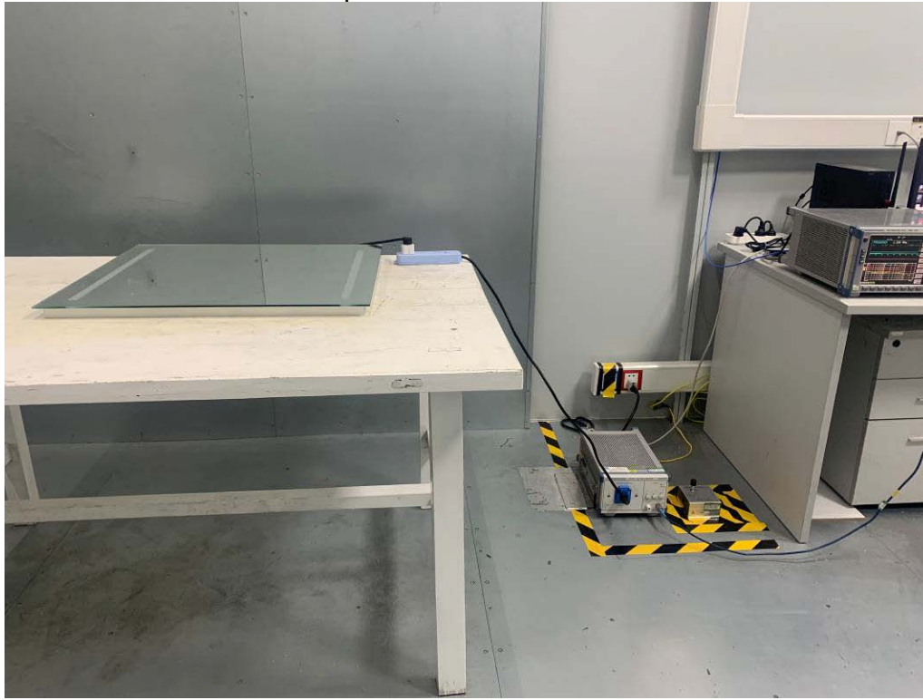
Photos of radiated emission test 30MHz – 1GHz
