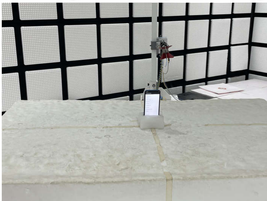
Radiated spurious emission Test Setup-2(Above 1GHz)
