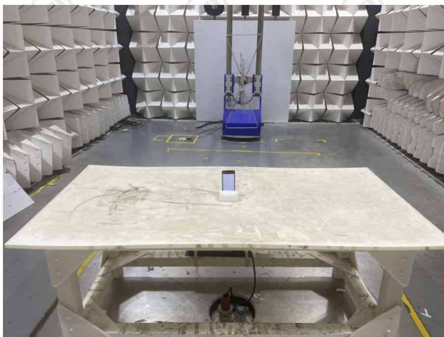
Radiated Spurious Emissions Test Setup (30MHz ~ 1GHz)
