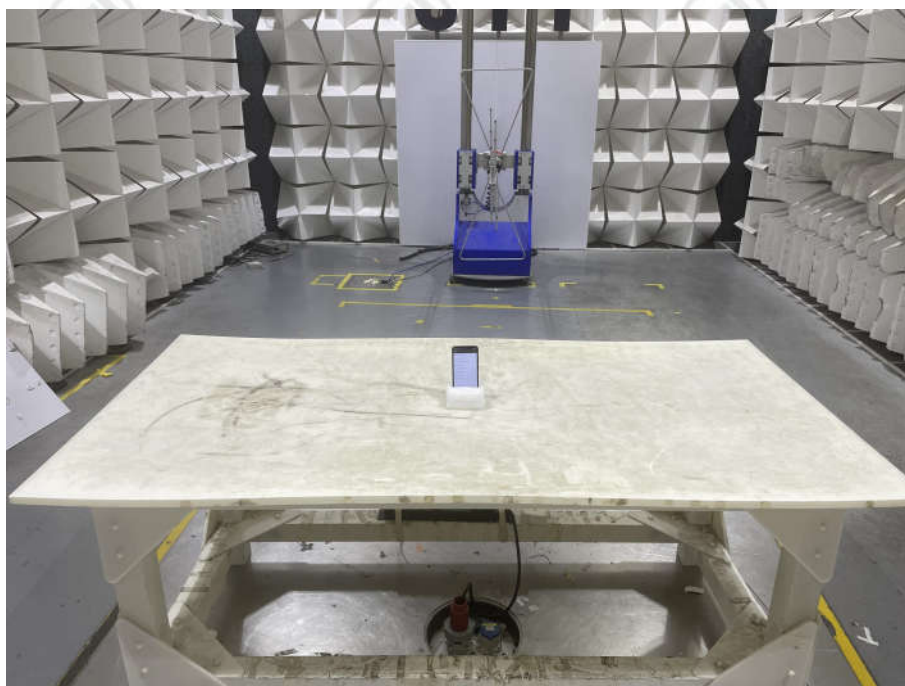
Radiated spurious emission Test Setup-1(Below 1GHz)
