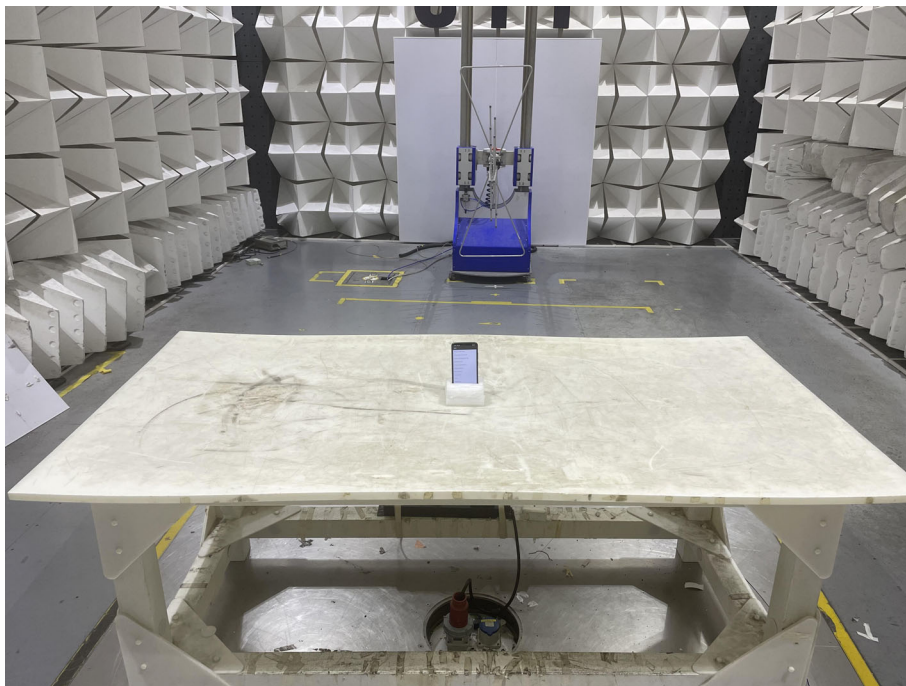
Radiated spurious emission Test Setup-1(Below 1GHz)
