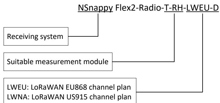
Flex2 transmitters are also shipped without the provisioning and the receiving system. For these versions, the user must manually configure the LoRaWAN radio parameters into the measurement module via USB. With this functionality, the effortless interchangeability of the measurement modules is lost.
