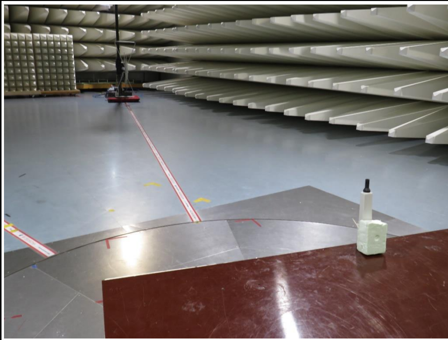
Test setup configuration 3 antenna VULB 9126 horizontal AC 6
