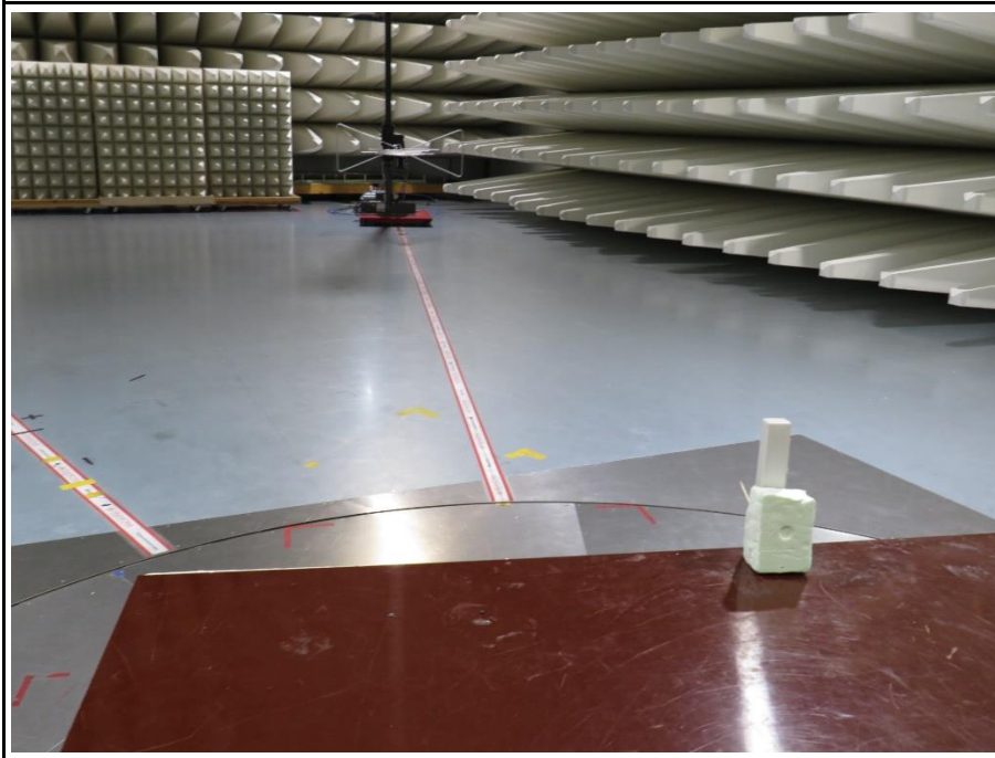
Test setup configuration 2 antenna VULB 9162 horizontal AC 6
