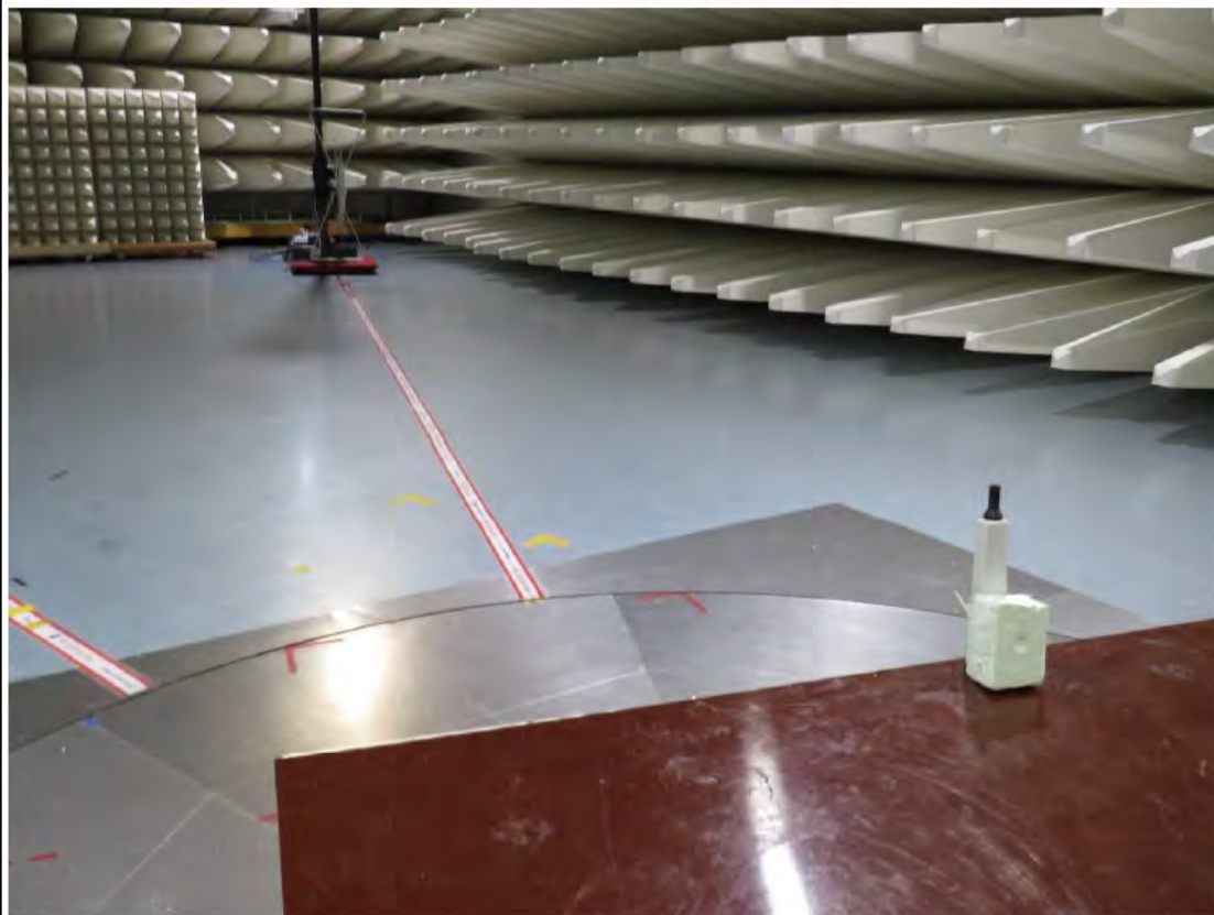
Test setup configuration 3 antenna VULB 9126 horizontal AC 6
