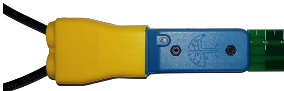
**Step 5 : slide cable seal into cap**
