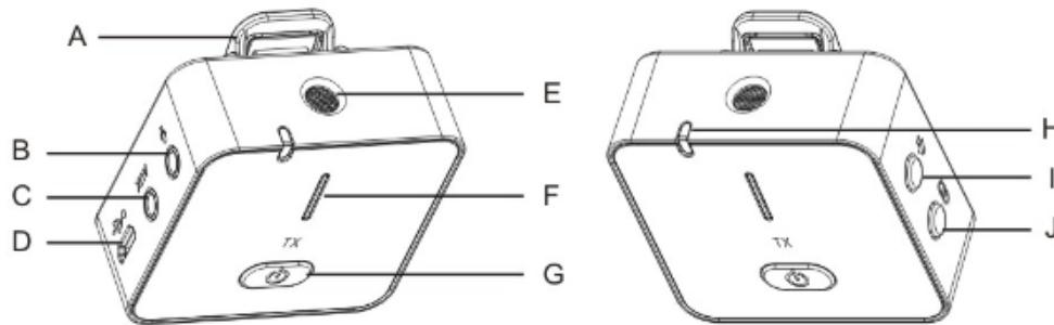
A: Fixing clip: can be quickly installed to the required fixed position.
