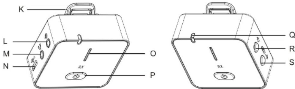
K: Fixing clip: can be quickly installed to the required fixed position.
