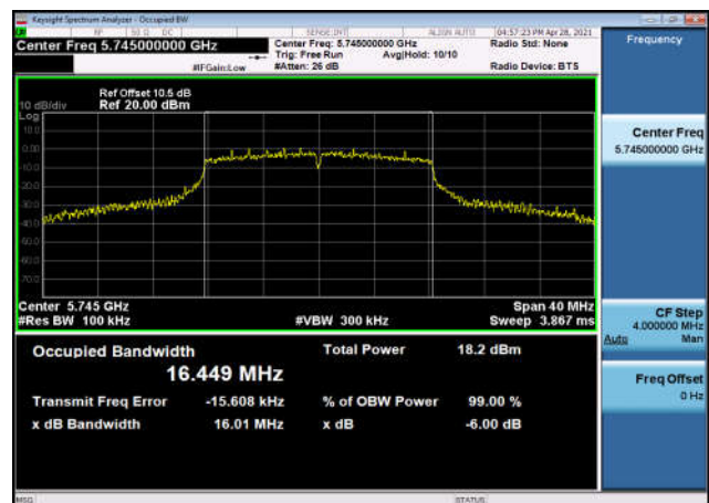
U-NII-3 6dB Bandwidth-802.11a(20MHz) ,5745MHz,Ant1
