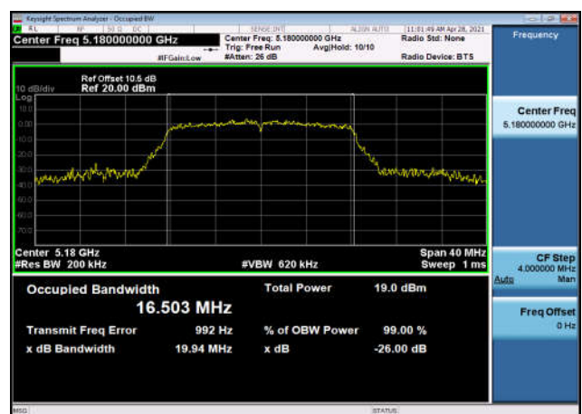
U-NII-1 26dB Bandwidth-802.11a(20MHz) ,5180MHz,Ant1
