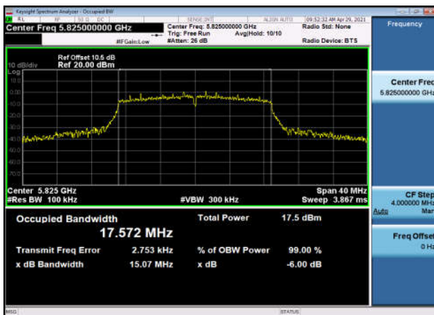
U-NII-3 6dB Bandwidth-802.11n(40MHz) ,5795MHz,Ant1
