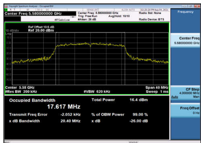
U-NII-2c 26dB Bandwidth-802.11n(20MHz ,5580MHz,Ant1
