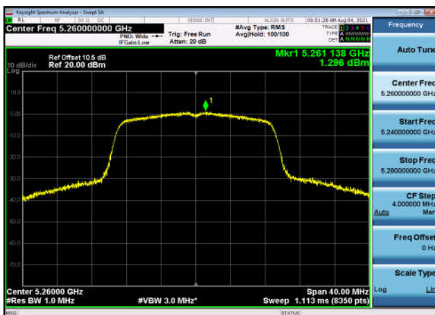
U-NII-2a Power spectral density-802.1 1ac(20MHz),5260MHz,Ant1
