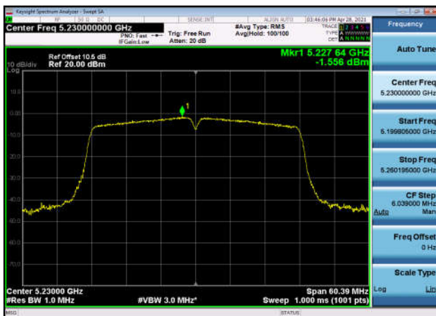
U-NII-2a Power spectral density-802.1 1n(20MHz),5260MHz,Ant1
