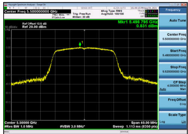
U-NII-2c Power spectral density-802.1 1a(20MHz),5700MHz,Ant1
