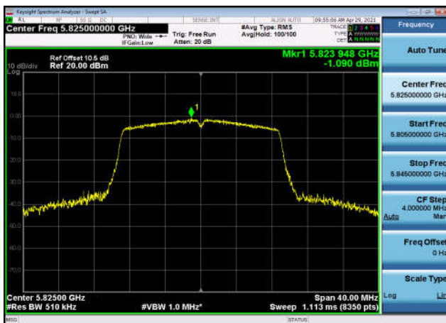
U-NII-3 Power spectral density-802.11 n(40MHz),5795MHz,Ant1
