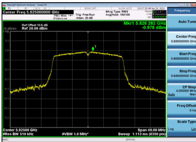
U-NII-3 Power spectral density-802.11 ac(20MHz),5825MHz,Ant1
