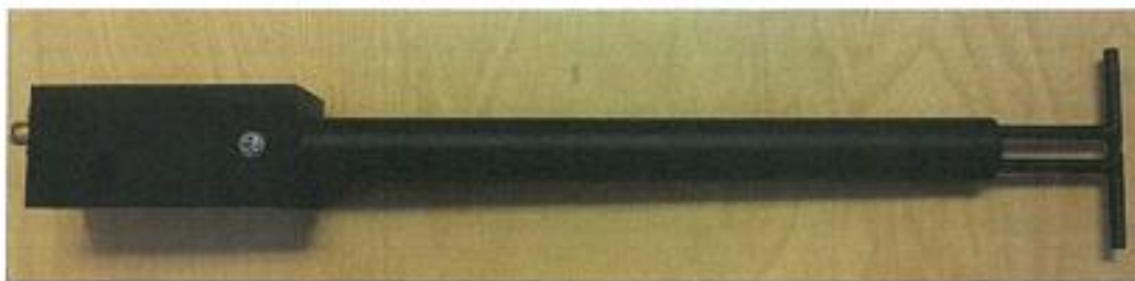
Figure 1 – MVG COMOSAR Validation Dipole
