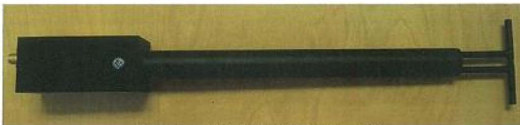
Figure 1 – MVG COMOSAR Validation Dipole
