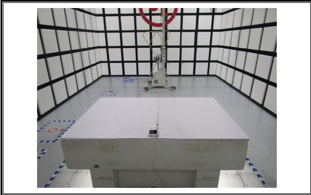
RADIATED RF MEASUREMENT SETUP (30MHz ~ 1 GHz)
