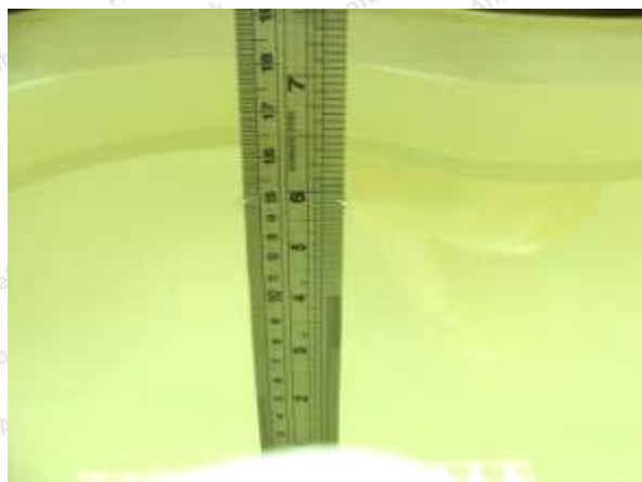
Photo of Liquid Height for Head SAR
