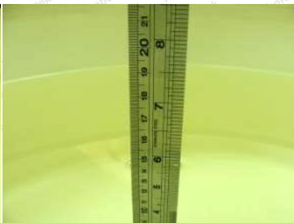
Photo of Liquid Height for Body SAR
