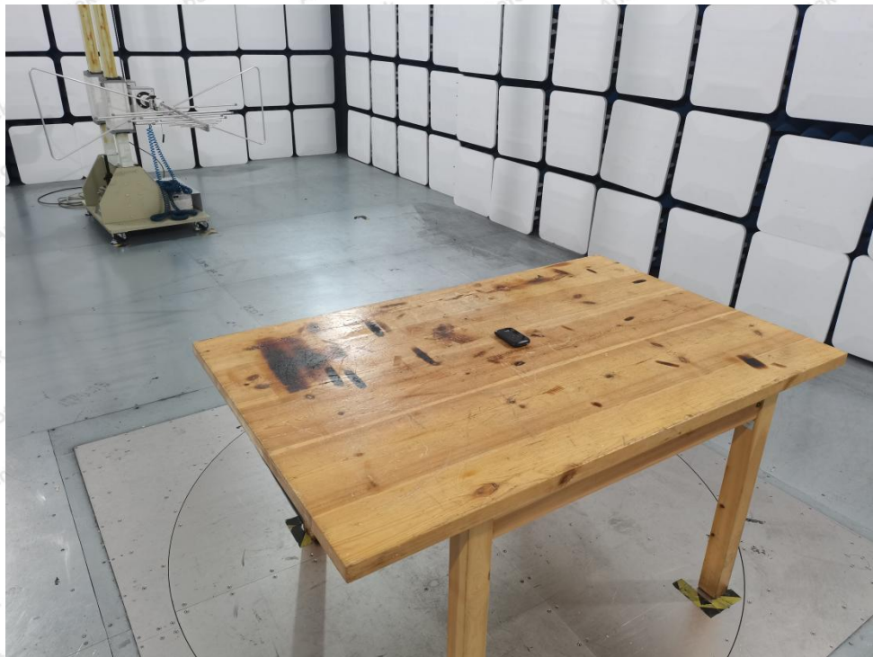
Photo of Radiation Emission Test
