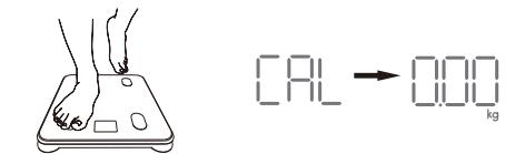
3. Step on the scale with 1 foot until digits appear on the display, then step off. The scale will show "CAL" while calibrating, then "0.0" when calibration is complete.
