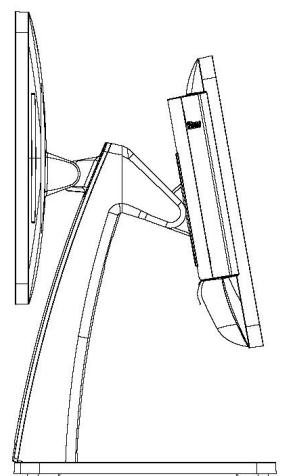
15.6-inch main screen + 15.6-inch secondary screen, length × width × height: 380mm\*205mm\*362mm; main screen flip angle 0-45°, secondary screen flip angle 0-30°
