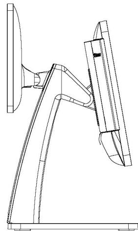
15.6-inch main screen + 10.1-inch secondary screen, length×width×height: 380mm\*205mm\*353mm; the flip angle of the main screen is 0-45°, and the flip angle of the secondary screen is 0-30°
