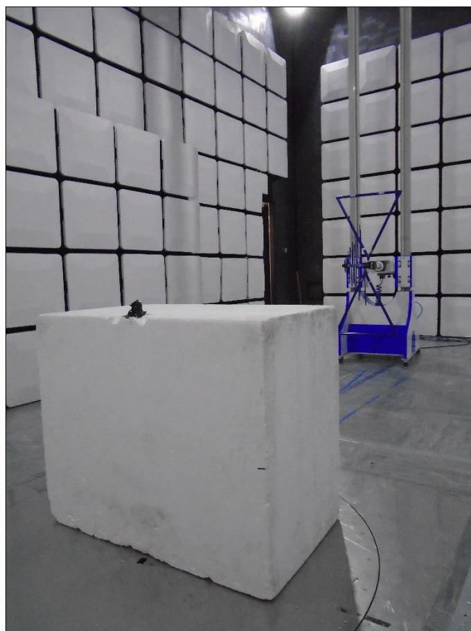
Figure 71 - Test Setup - 30 MHz to 1 GHz Orientation Y
