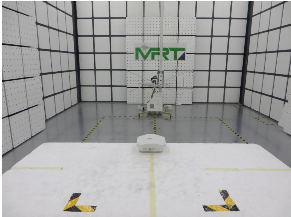
Description: Radiated Spurious Emissions Test Setup for above 1GHz\_2<sup>nd</sup> model
