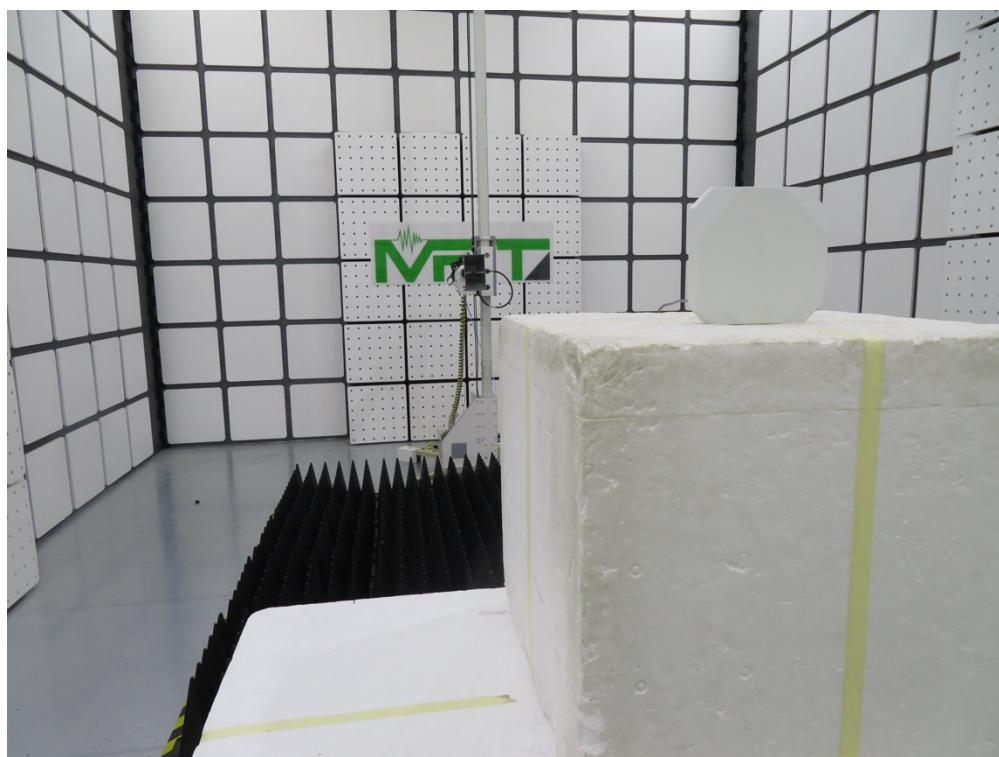
Description: Radiated Spurious Emissions Test Setup for below 1GHz\_2<sup>nd</sup> model
