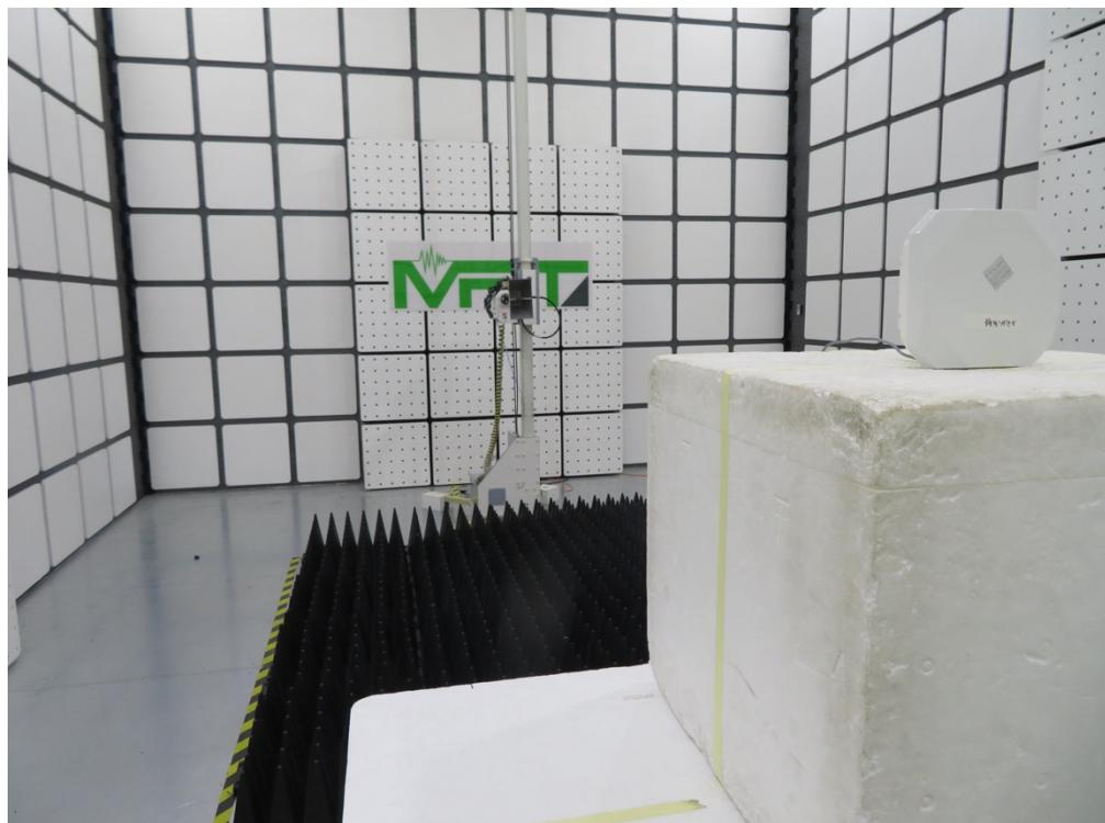
Description: Radiated Spurious Emissions Test Setup for below 1GHz\_3<sup>rd</sup> model
