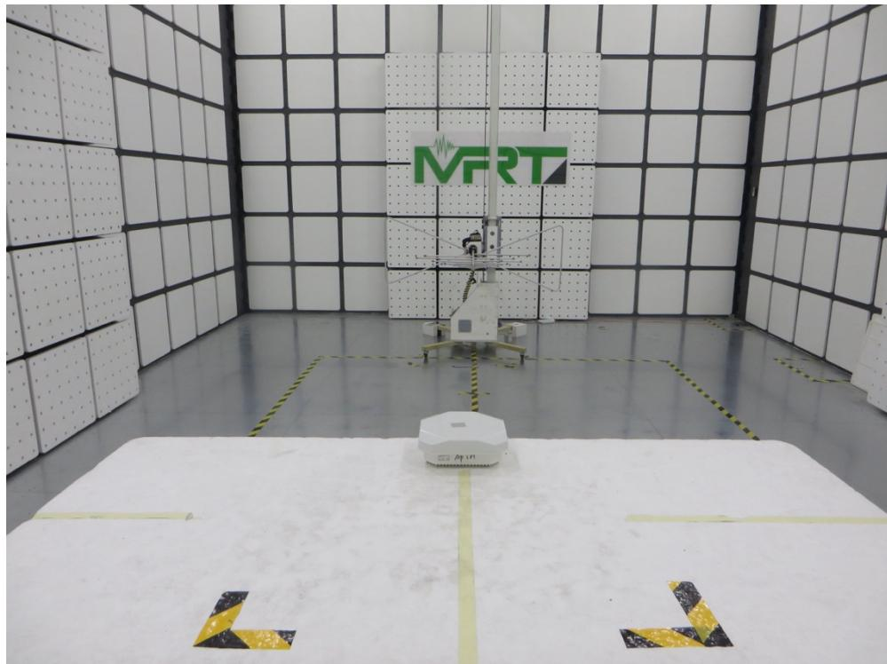
Description: Radiated Spurious Emissions Test Setup for above 1GHz\_1<sup>st</sup> model
