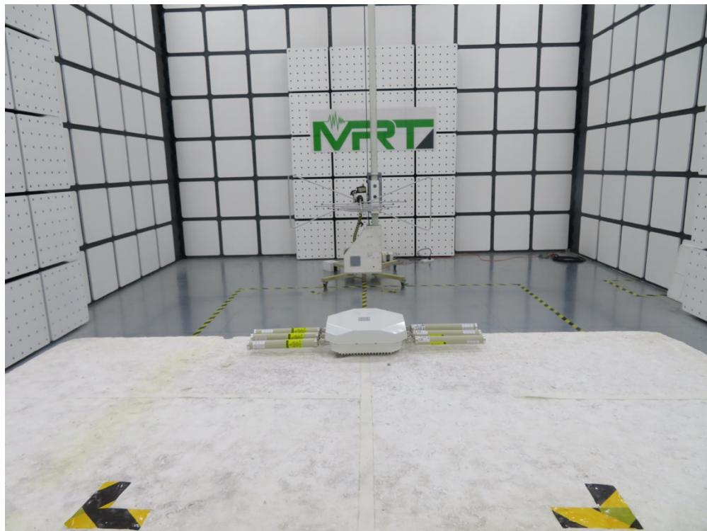
Description: Radiated Spurious Emissions Test Setup for above 1GHz\_3<sup>rd</sup> model
