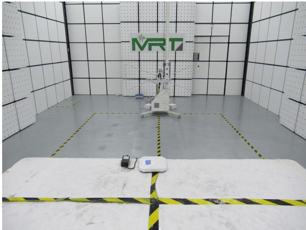
**Test Mode 1****Description: Front View of Radiated Emission Test Setup (1 ~ 18GHz)**
