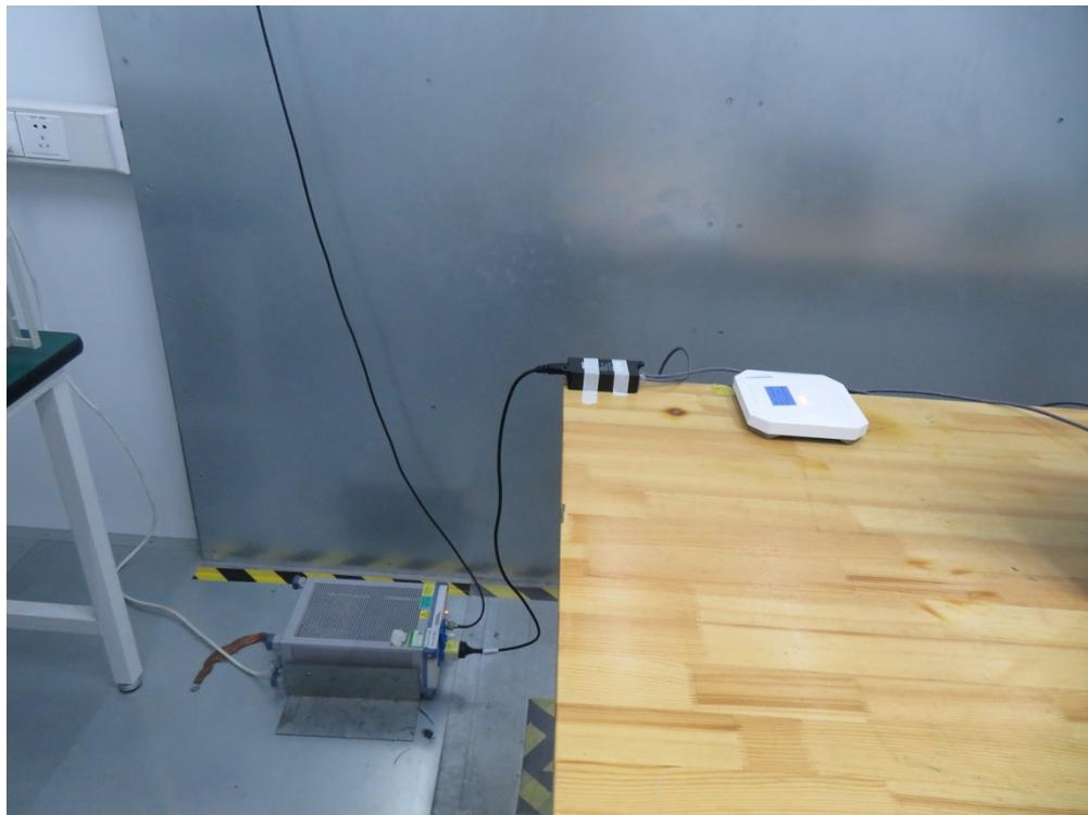
**Test Mode 2****Description:** Back View of Conducted Emission Test Setup for Power Port
