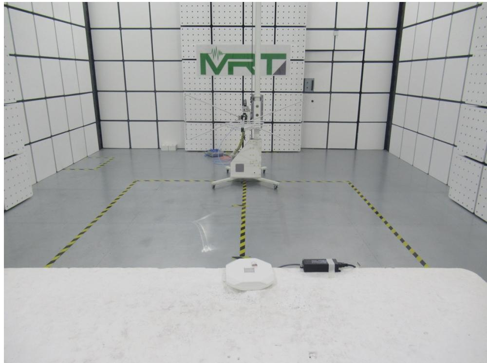
**Test Mode 2****Description: Radiated Emission Test Setup (1GHz ~ 18GHz)**
