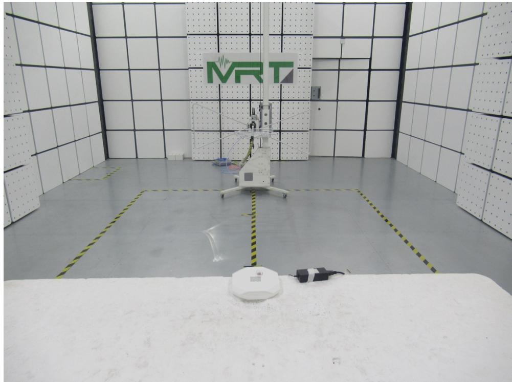
**Test Mode 1****Description: Radiated Emission Test Setup (1GHz ~ 18GHz)**
