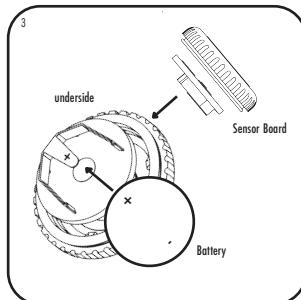
EN: Battery placed on underside of device board. Providing power to the unit.
