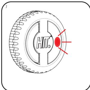
EN: Device will continue to record and store IMPACT data until you stop recording on app or turn off device. When device flashes RED the device has registered a G-Force impact over the traffic light threshold.
