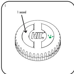
EN: To turn on device, push and hold the button segment of the IMPACT device for 1 second. The device will flash green then flash consistently to confirm ready state.
