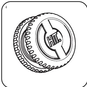
EN: Push device back together with finger and forethumb (you may need to use both hands). The device is sealed when the top cap 'clicks' into place with the bottom cap. The device is now sealed and water resistance.
