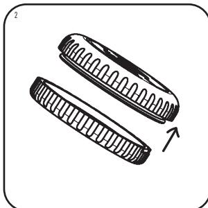
EN: To open Device use a finger nail to prise device seal apart.
