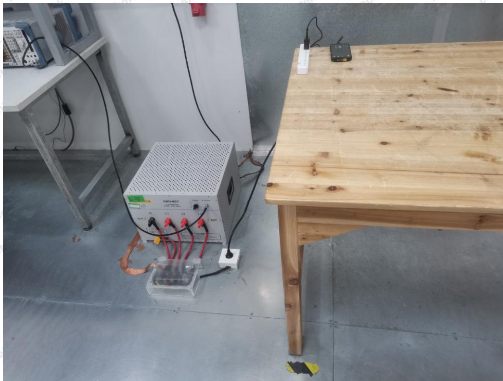
Photo of Conducted Emission Measurement
