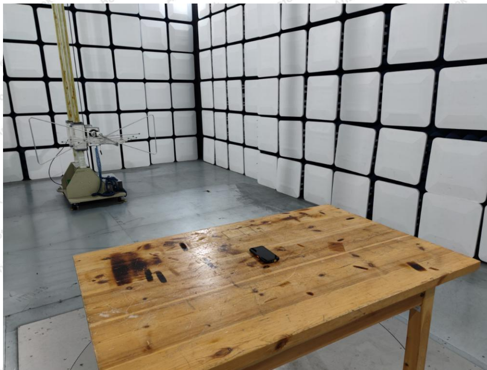
Photo of Radiation Emission Test
