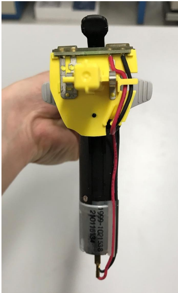
Figure 10: PCBA Battery Bulkhead and Contacts Close Up
