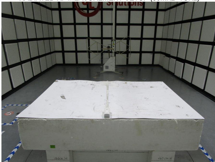
RADIATED RF MEASUREMENT SETUP (30MHz~1GHz)
