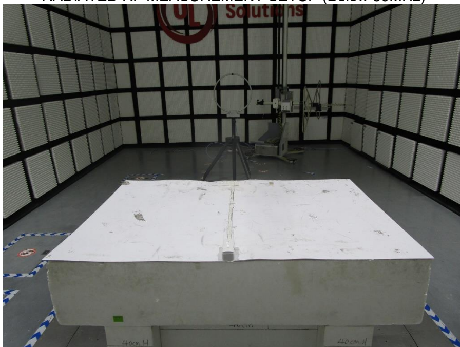
RADIATED RF MEASUREMENT SETUP (Below 30MHz)
