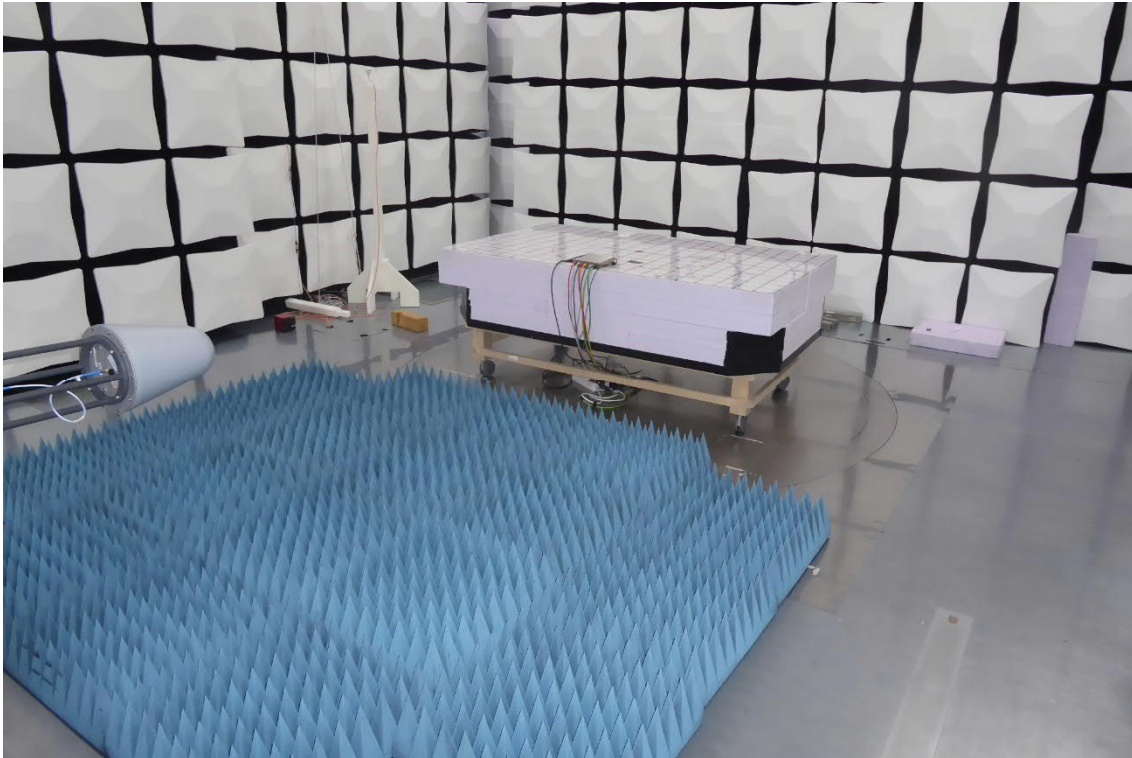
Test setup 5: Radiated Emission/1 GHz - 12 GHz
