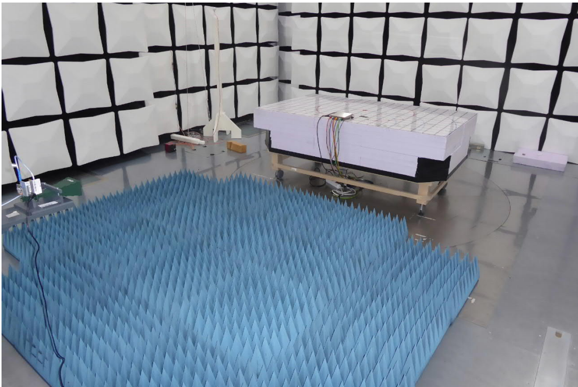
Test setup 6: Radiated Emission/12 GHz - 18 GHz
