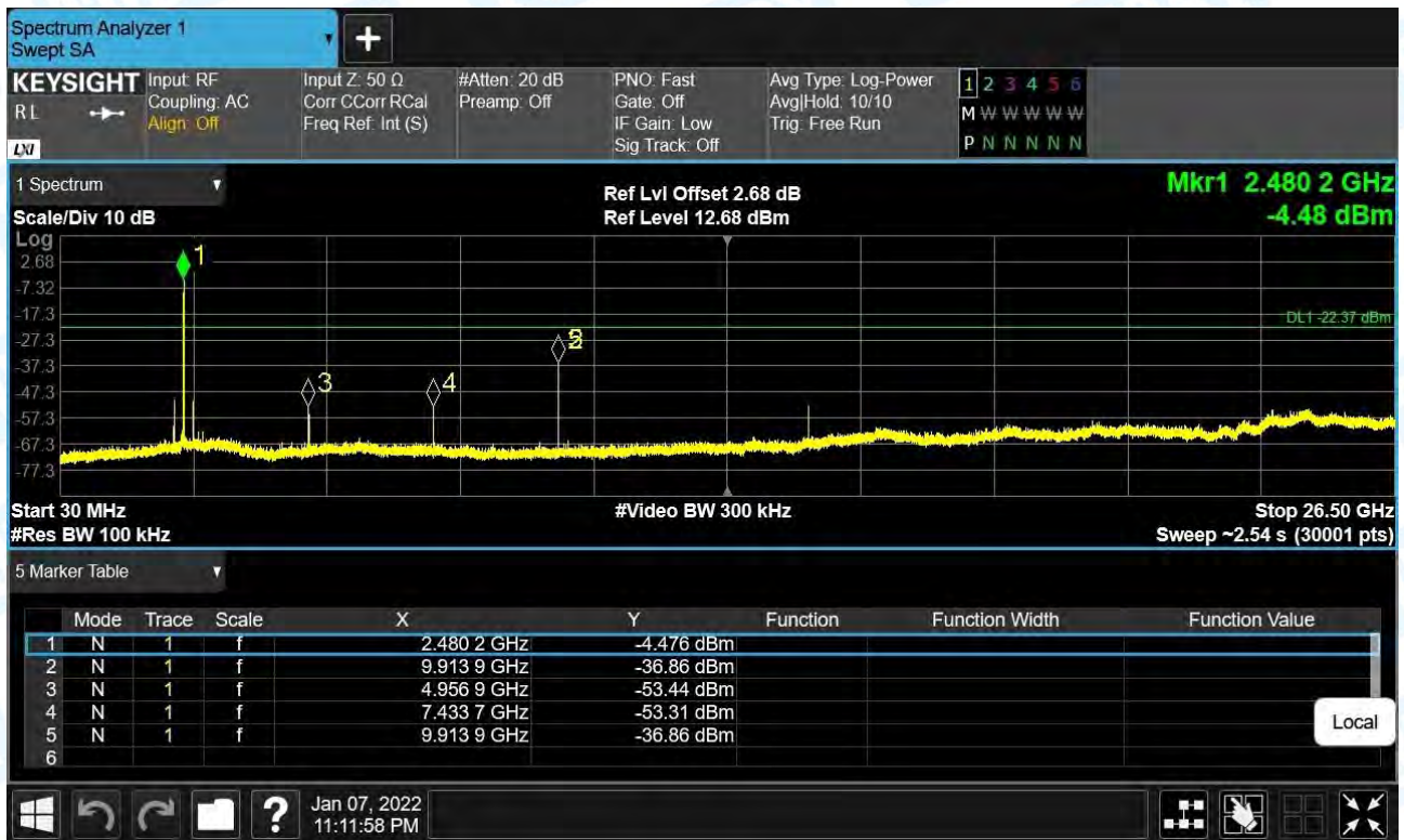
Tx. Spurious NVNT 1-DH1 2480MHz Ant1 Emission
