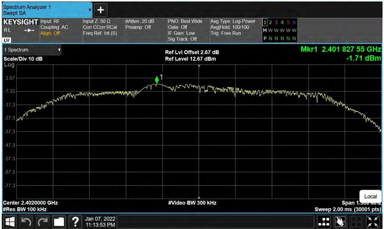
Tx. Spurious NVNT 2-DH1 2402MHz Ant1 Emission
