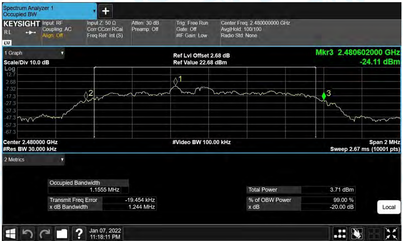
-20dB Bandwidth NVNT 2-DH1 2480MHz Ant1
