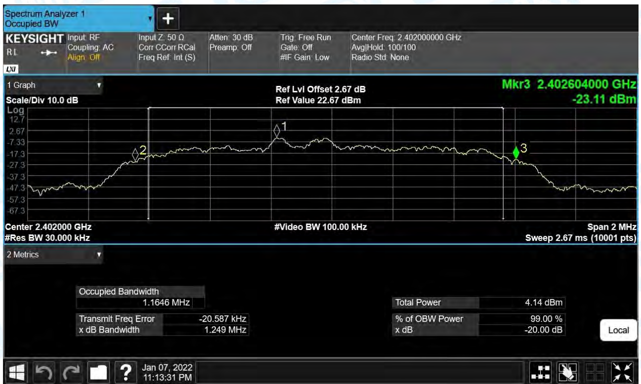
-20dB Bandwidth NVNT 2-DH1 2402MHz Ant1
