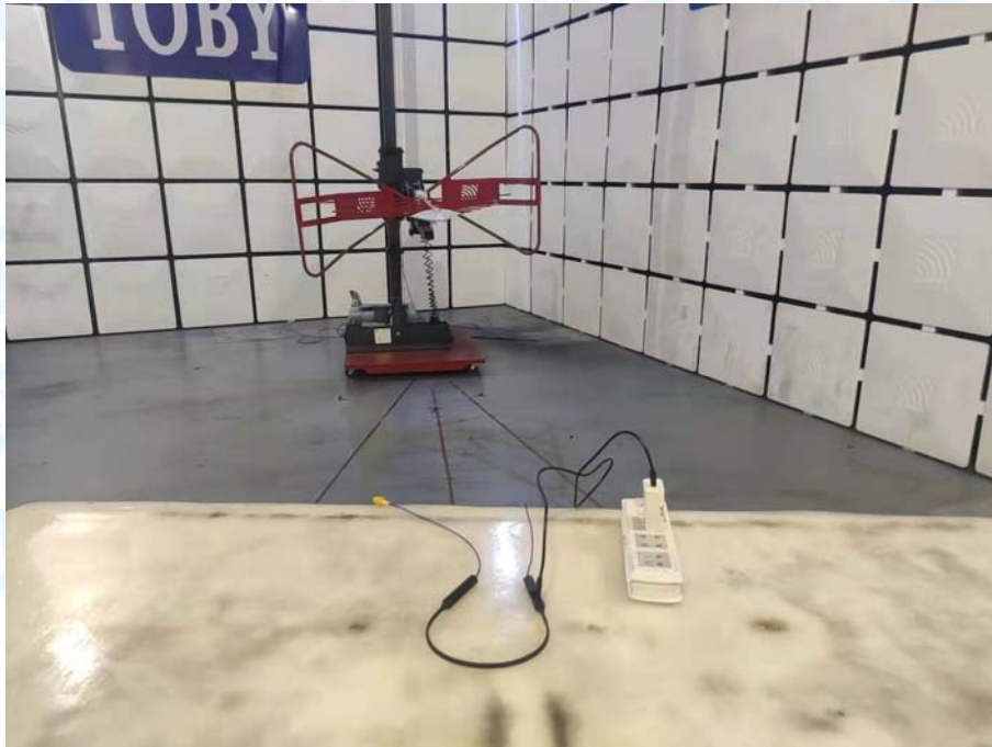
Photo of Setup for Conducted Emission
