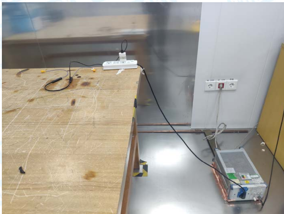
Photo of Setup for Conducted Emission
