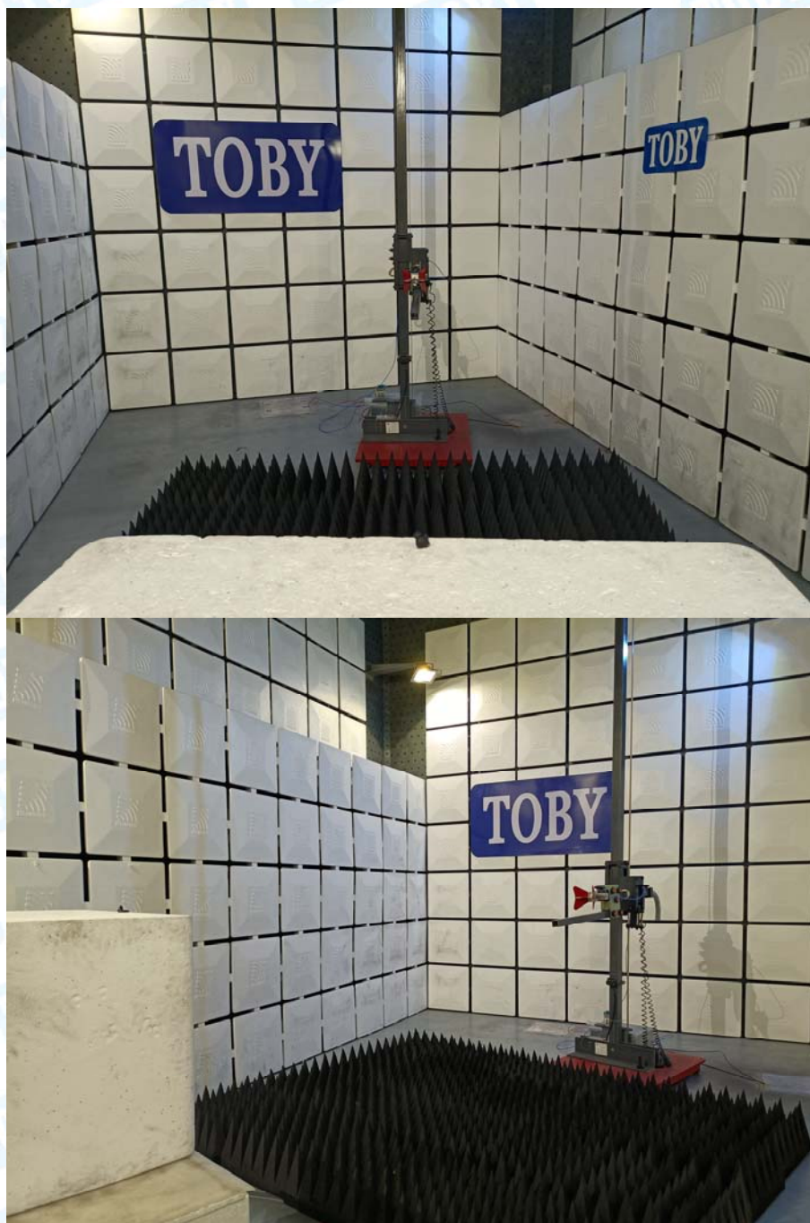
Photo of Setup for Radiated Emission (Above 1 GHz)
