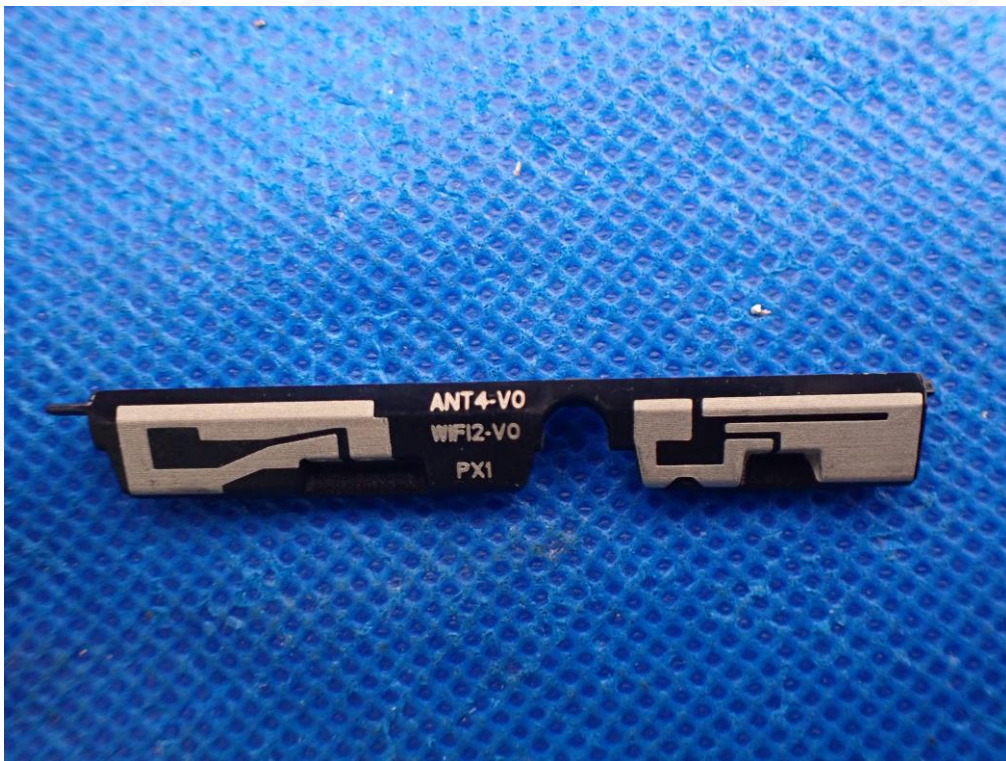
LTE:1/3/41 DRX_MIMO& n1/n3/n41 RX3 ANTENNA
