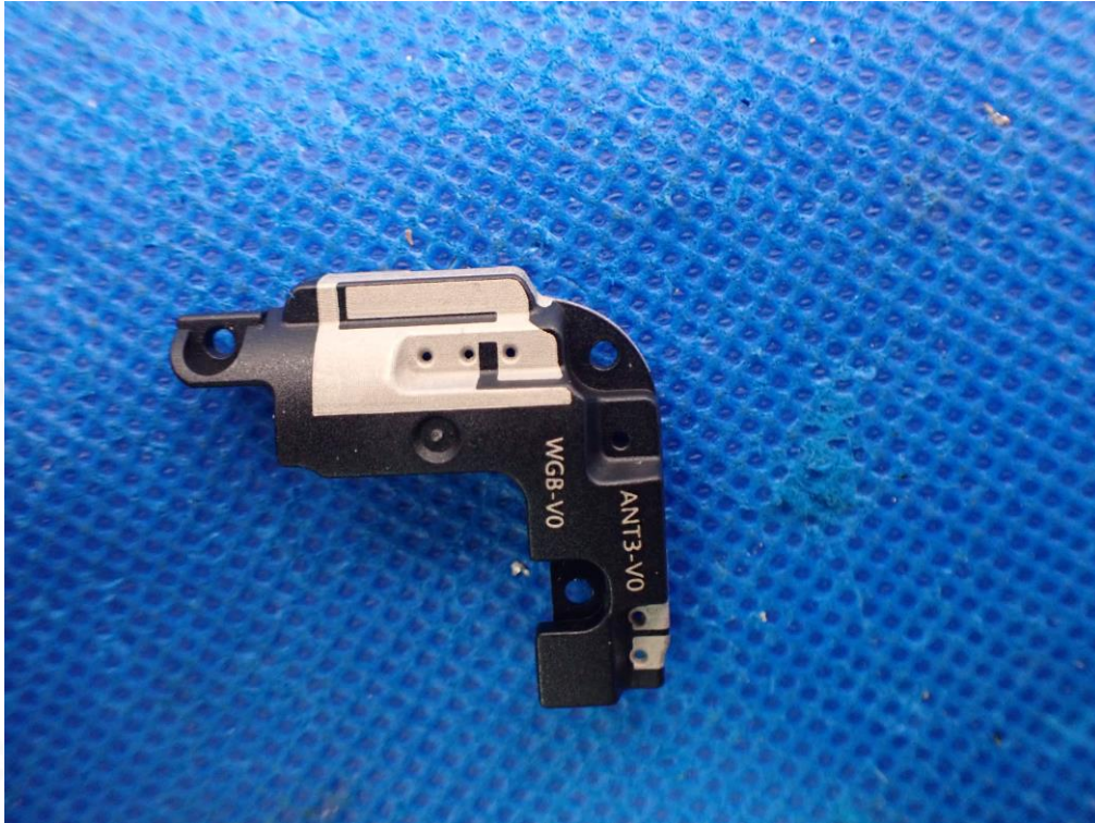
LTE:1/3/41 DRX_MIMO& n1/n3/n41 RX3 ANTENNA
